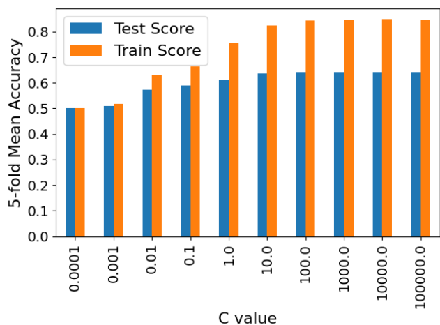
Figure 3: Grid search for C parameter for logistic regression on TF-IDF embeddings using 5-fold validation. X-axis: Value for parameter C, the inverse of the regularization coefficient. Y-axis: Mean accuracy on the validation set (blue) and the testing set (orange).
