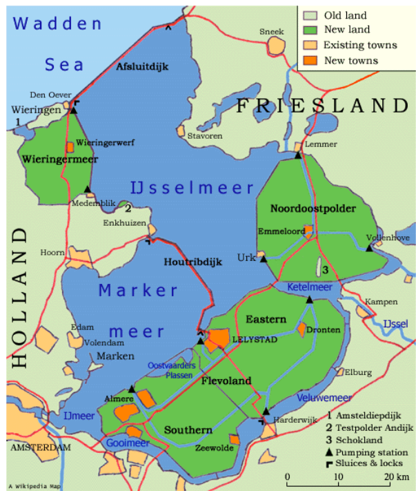
Figure 1.4: Map of the Zuiderzee works where lake IJsselmeer and lake Markermeer are created (www.wikipedia.org).
