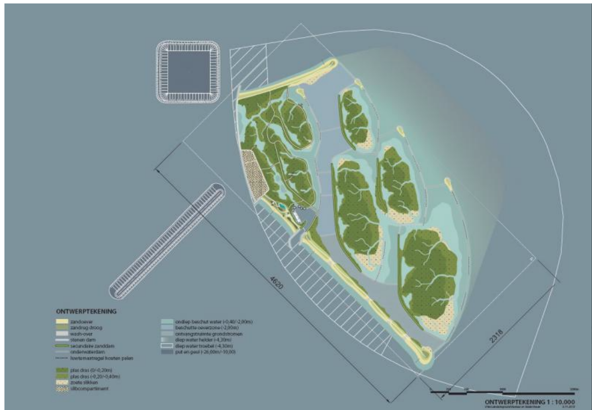
Figure 1.5: Design of the Marker Wadden project with a borrow pit in the north and silt trap in the east [Geretsen, 2014]. Sand dams provide protection against wave attack and enclose areas to trap deposited mud. Behind the sand dams a marsh-pond habitat is created that is attractive for birds.
