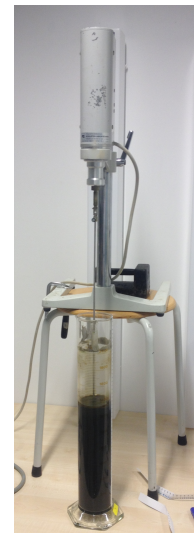
Figure 3.3: Vane test set-up rotovisco measuring system Haake M1500.
