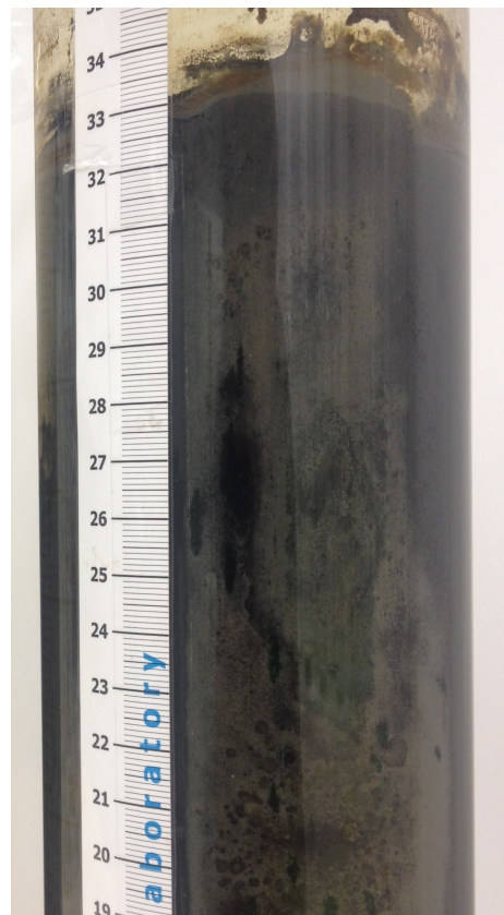
Figure 4.23: Settling column experiment t=97 days. During the SIC300 test there was no exposure to light which led to almost no organic growth in the column.
