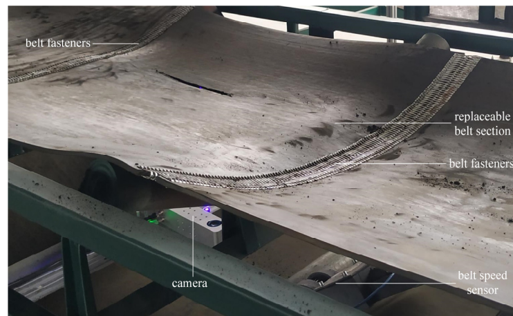
Figure 8. The simulation experiment platform in laboratory; only the replaceable belt section needs to be replaced rather than the whole belt in each experiment.
