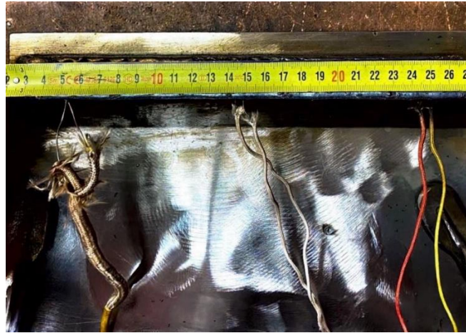
Figure 11: Thermocouple connection to a WAAM print
