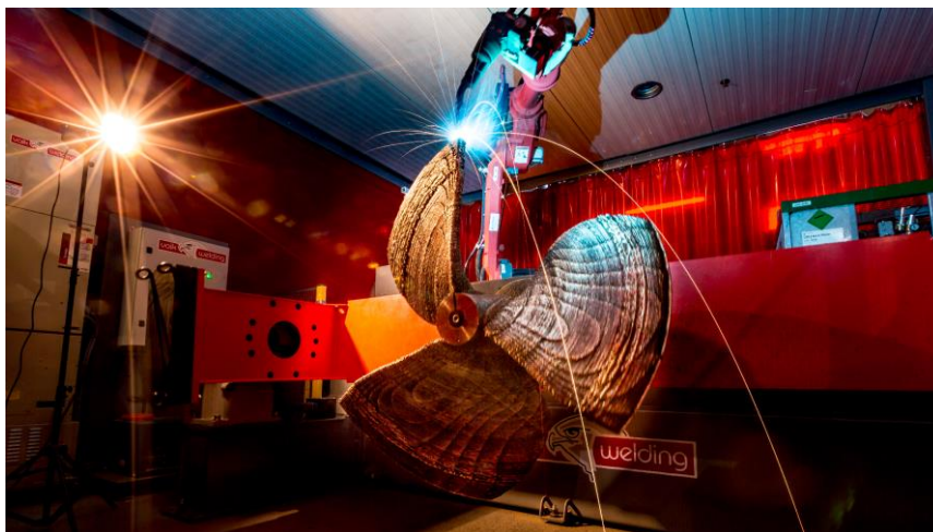
Figure 1: Depiction of WAAM, courtesy RAMLAB
