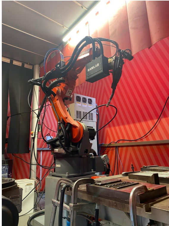
Figure 10: Panasonic TM1400 WGIII robot used for printing experiments
