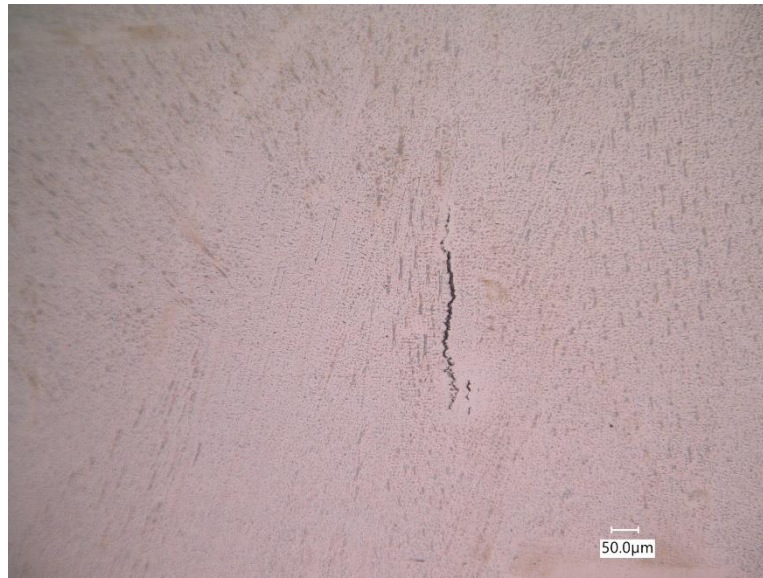
Figure 5: Microscopic solidification cracks in repair material samples
