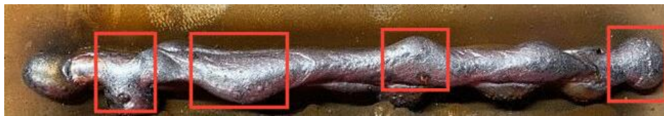
Figure 14: Invar 36 bead with irregularities caused by bead overflow (superactive mode, 15.6V, 0.25 m/min travel speed)
