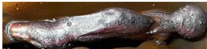
Figure 47: Invar 36 bead showing overflow
