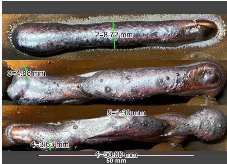
Figure 36: Unacceptable (3, 4) and acceptable (5) overflow defects seen in Invar 36 beads
