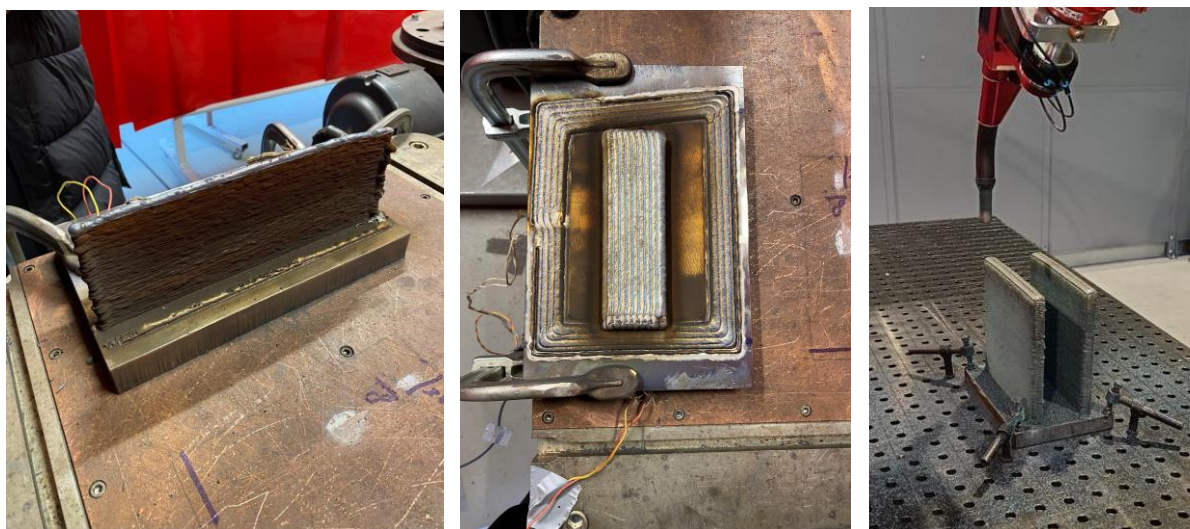
(a) (b) (c) Figure D4a-c: Large samples of (a) Invar 36, (b) Inconel 718, (c) Inconel 625
