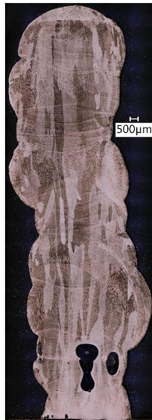
Figure 40: Significant porosity seen in a single-bead-thickness wall of Invar 36
