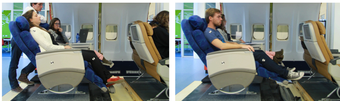
Figure 6.8 | Subject watching IFE in slouched posture while A) deorsumducting the eyes by contracting a.o. the m. inferior rectus and m. inferior oblique B) flexing the head forward with respect to the trunk by contracting a.o. the m. sternocleidomastoid (from Smulders et al. (2016))
