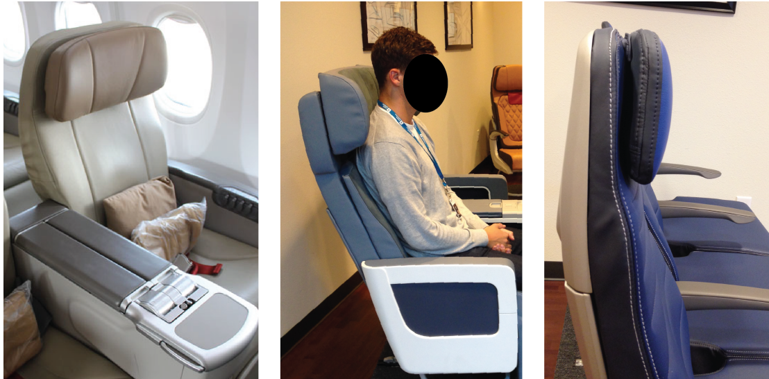
Figure 4.9 | Left: Virgin Australia domestic-business class seat with protruding headrest. Middle: Z600 domestic-business class seat with protruding headrest. Right: an ZSUS economy class seat where the headrest has a slimmer profile as the backrest provides an indented space.
