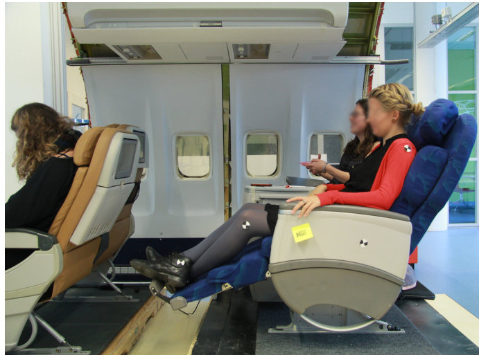
Figure 13.1 | Test setup of IFE inclination test
