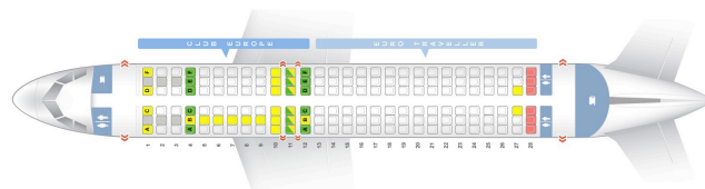
Figure 4.3 | LOPA narrow body single aisle, two class British Airways Airbus A320 European (TripAdvisor LLC, 2018)
