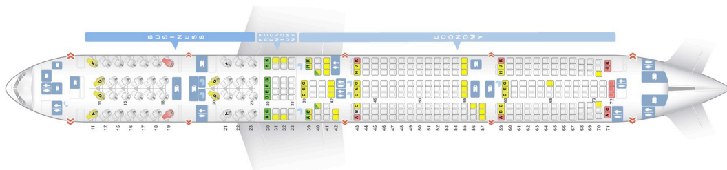
Figure 4.1 | LOPA wide body twin aisle, three class Cathay Pacific Boeing 777-300ER (TripAdvisor LLC, 2018)
