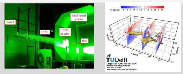
**Figure 1.** Tomographic PIV experiment with HFSB on a vertical axis wind turbine. Left: setup of the experiment. Right: flow field downstream of the blade tip. Experiments conducted at the open jet facility (OJF) of TU Delft.
