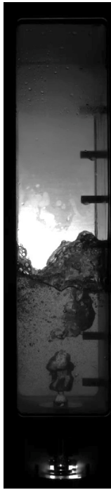
Fig. 15. Flow behavior inside the header with a 23 mm vertical upward feeding tube at a quality of x = 0.33 and total mass flux of G = 570 \text{ kg/(s m}^2\text{)} .
