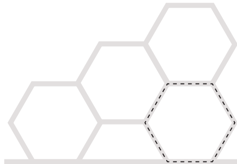
FIGURE 19 // Demarcation for each cell is halfway its thermal bridges
