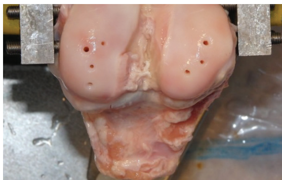
Figure 3. Drilled holes in porcine femora using water jets with various nozzle diameters.
