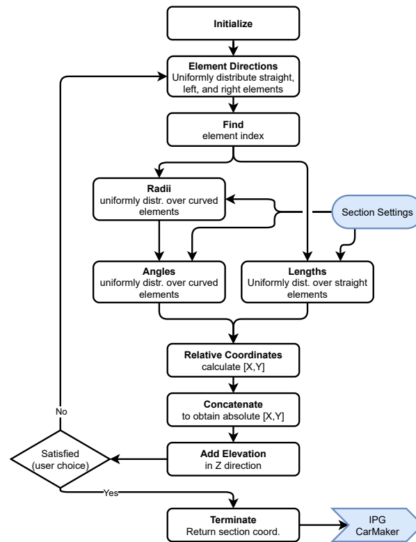
Figure B.1: Flowchart illustrating the generation of new highway section coordinates.
