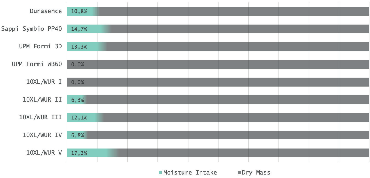
◀ Figure 48: Moisture Intake/ Measured difference in weight after submersion in water of different samples.
