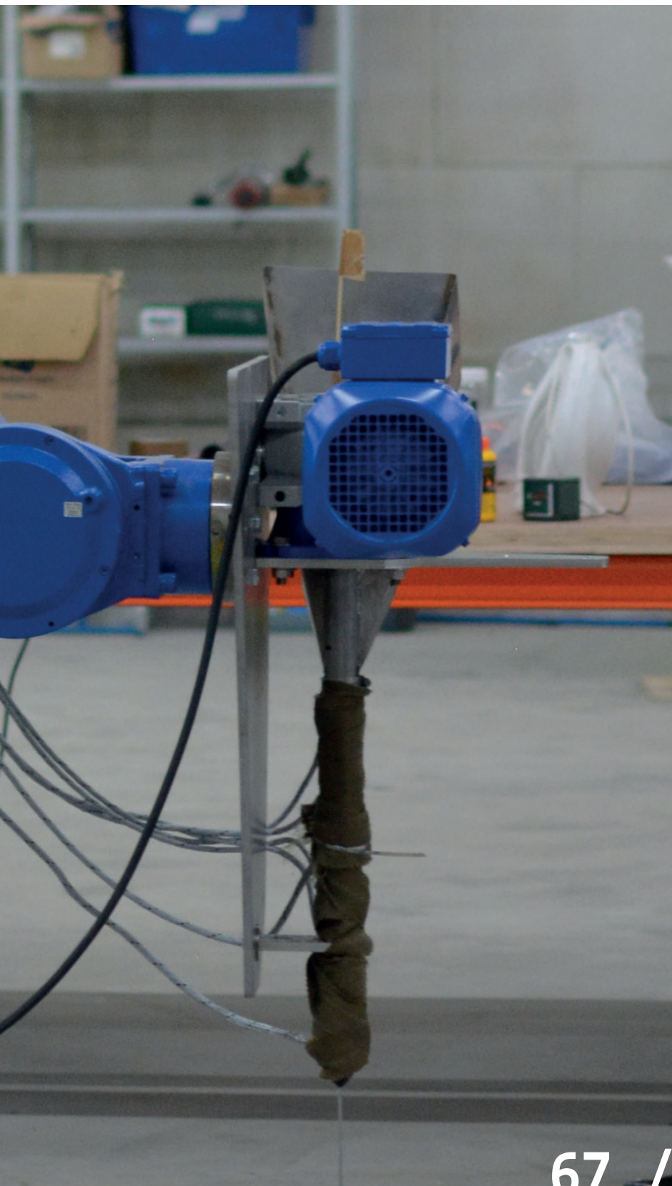
Figure 67: New Extruder (A3)/ ▼ Smaller extruder mounted on a robot for test printing.
