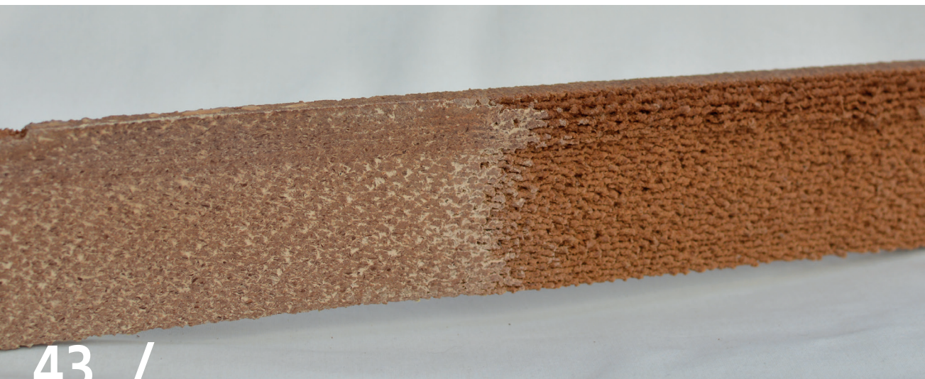
◀ Figure 43: Smooth Surface Print/ WFPP partly sanded down with an eccentric sander and grain P800.
