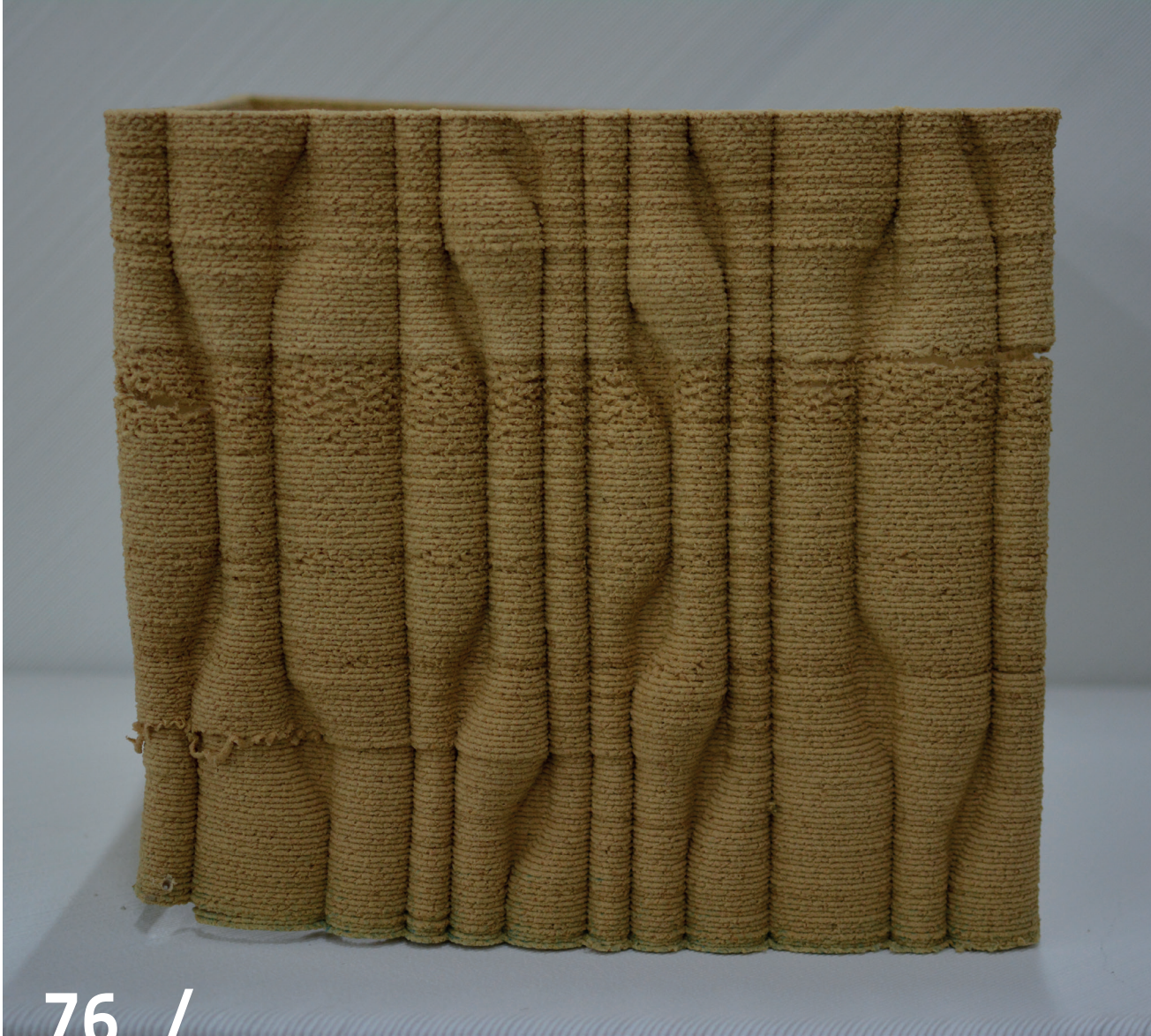
Figure 76: Test cube V_2/ ► New print with 50/50 Mixture material of CFPP and WFPP, printed with 4mm nozzle and double layer height compared to previous print.
