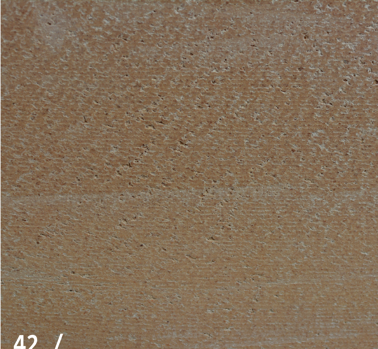
◀ Figure 42: Smooth Surface Print/ 50/50 mixture sanded down with an eccentric sander and grain P800.
