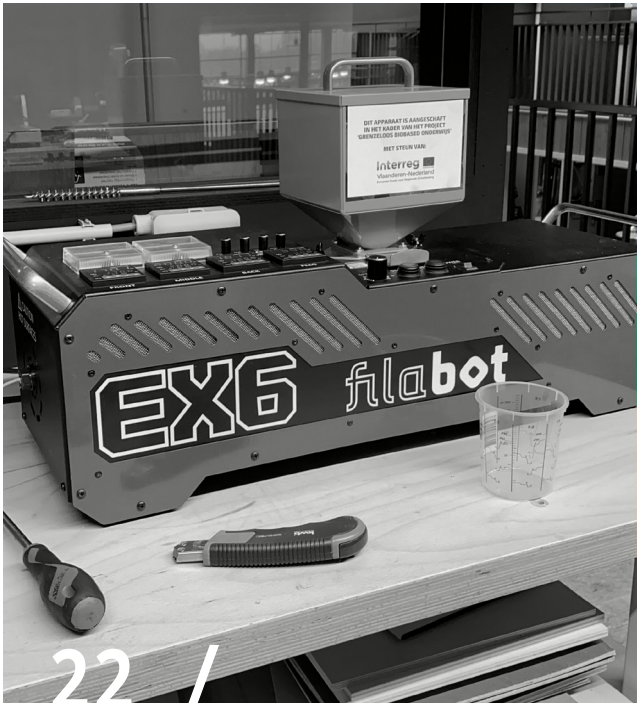
Figure 22: Filabot EX6 Estruder/ ▶ Lab extruder with more power and multiple heating zones for better extrusion performance.
