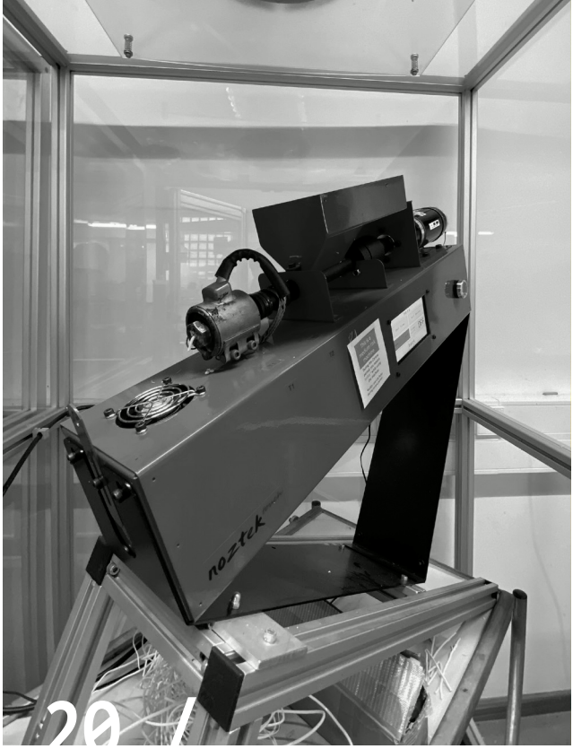
Figure 20: Noztek Pro Extruder/ ▶ Small lab extruder used for initial extrusion tests.
