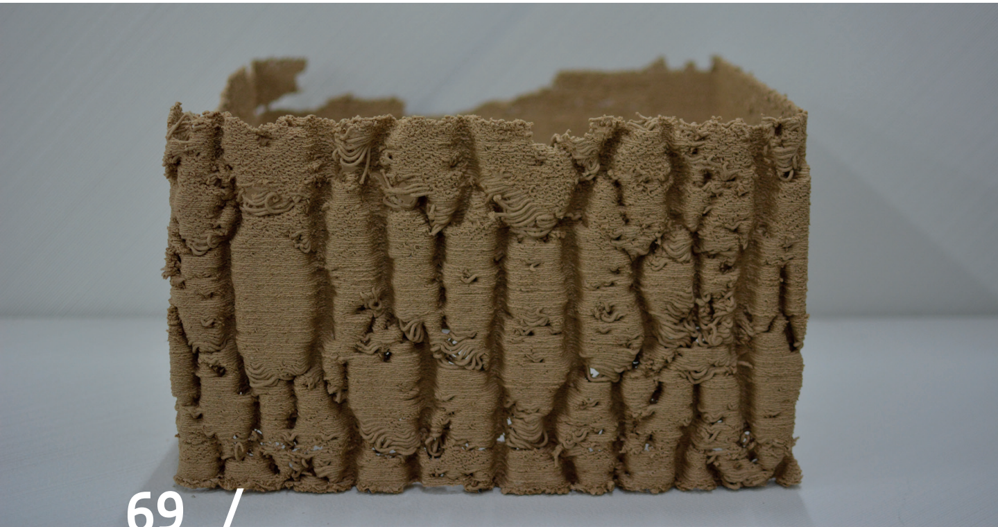
Figure 69: Test cube V_1/ ▲ First printed cube from 10XL/WUR batch II compound material and 2mm nozzle.
