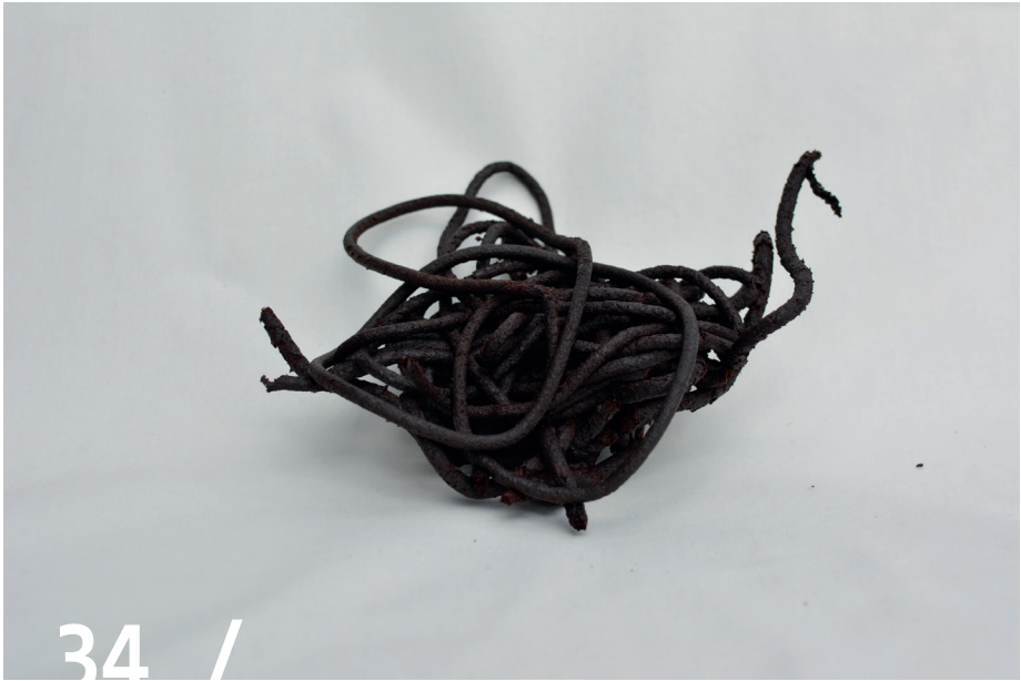
▼ Figure 34: UPM Formi WB60/ Heated too much, starting to char but showing a smooth surface.
