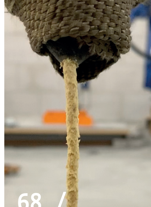
▲ Figure 68: Extrudate on A3/ The first extrudate on the new extruder (A3). Material: 50/50 mixture of WFPP and CFPP.
