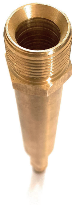
Figure 61: Brass Nozzle/ Shape of the nozzle used in the test setup.
