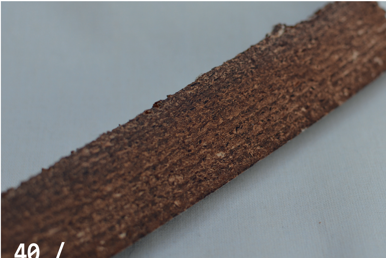
Figure 40: Smooth Surface Print/ ► WFPP sanded down with an eccentric sander and grain P800.
