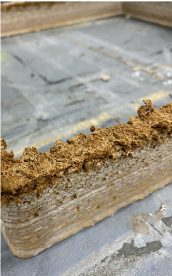
Figure 37: Rough Surface/ ▼ Representation of the fracturing of the surface for different materials when printing (50/50 mixture and WB60).
