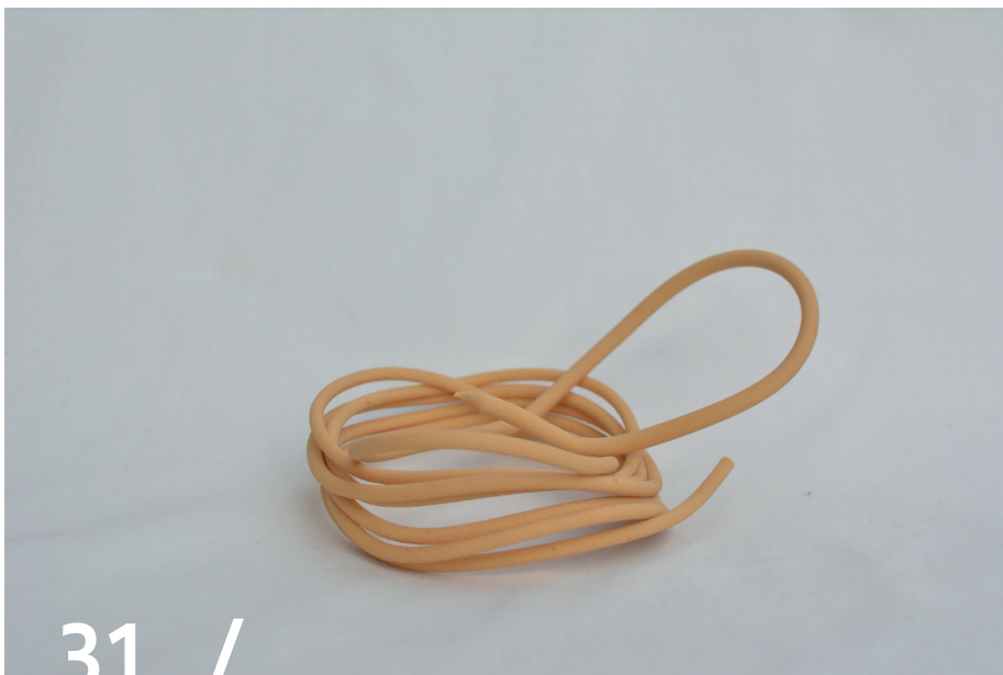
Figure 32: UPM Formi WB60/ ▲ Extrudate showing a rough and inconsistent surface.
