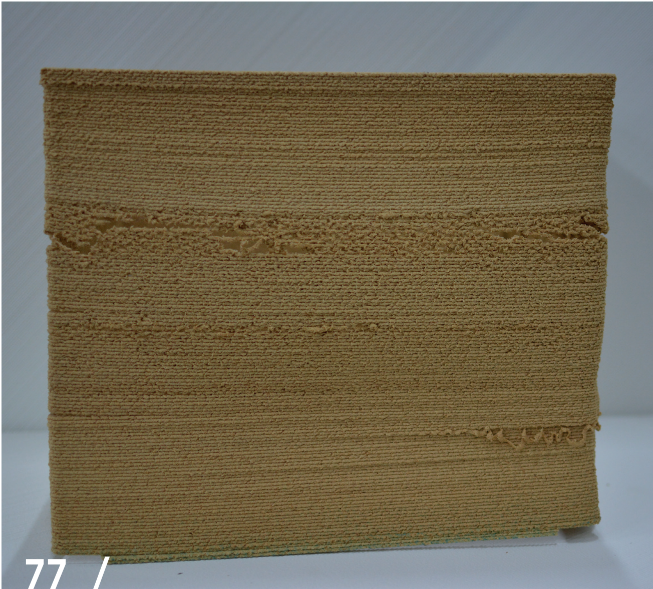
Figure 77: Flat wall of cube/ ► Print failures still an issue in this print, showing under extrusion and warping.
