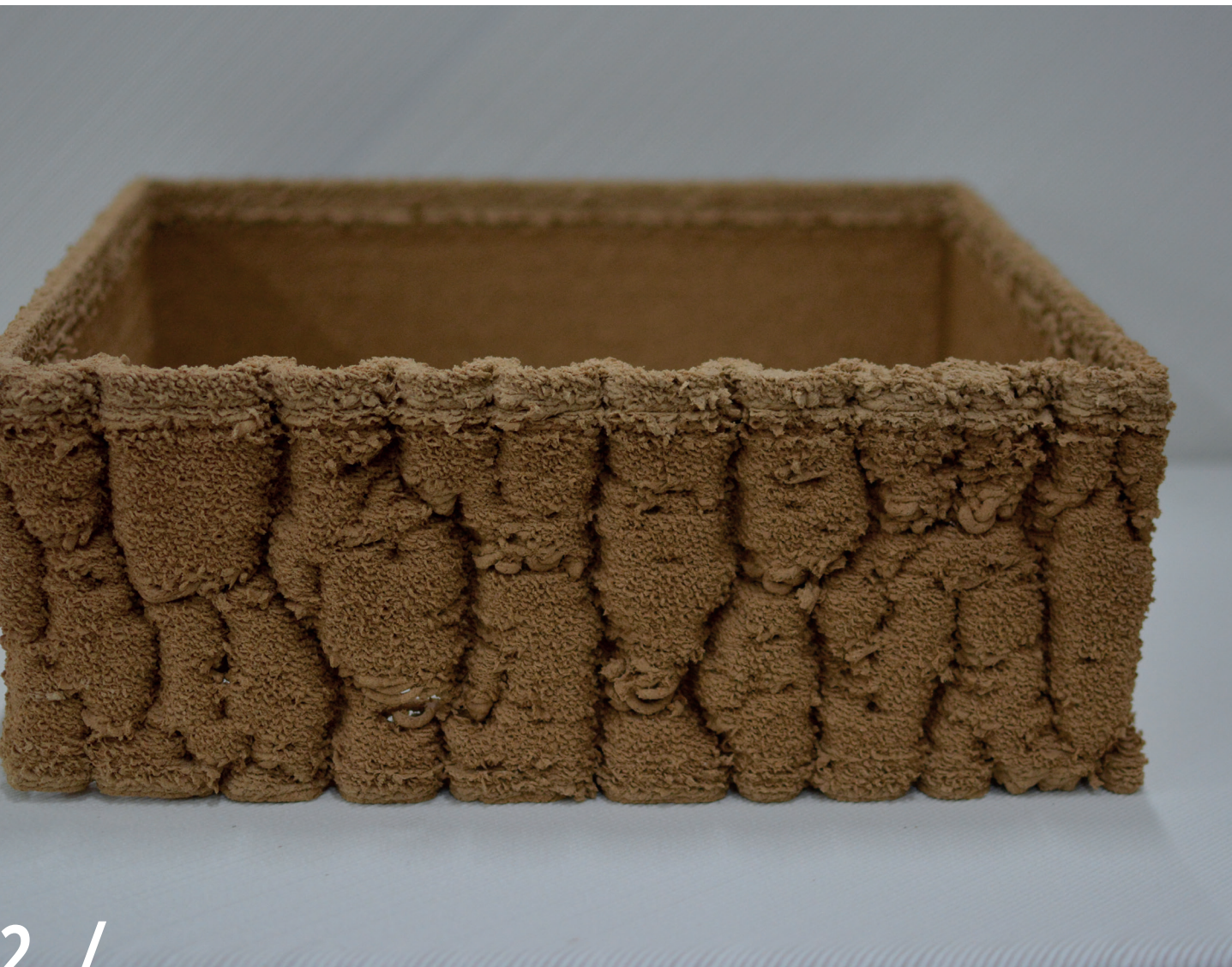
◀ Figure 72: Test cube V_1/ Partly printed cube with 10XL/WUR batch IV and a 4mm nozzle.
