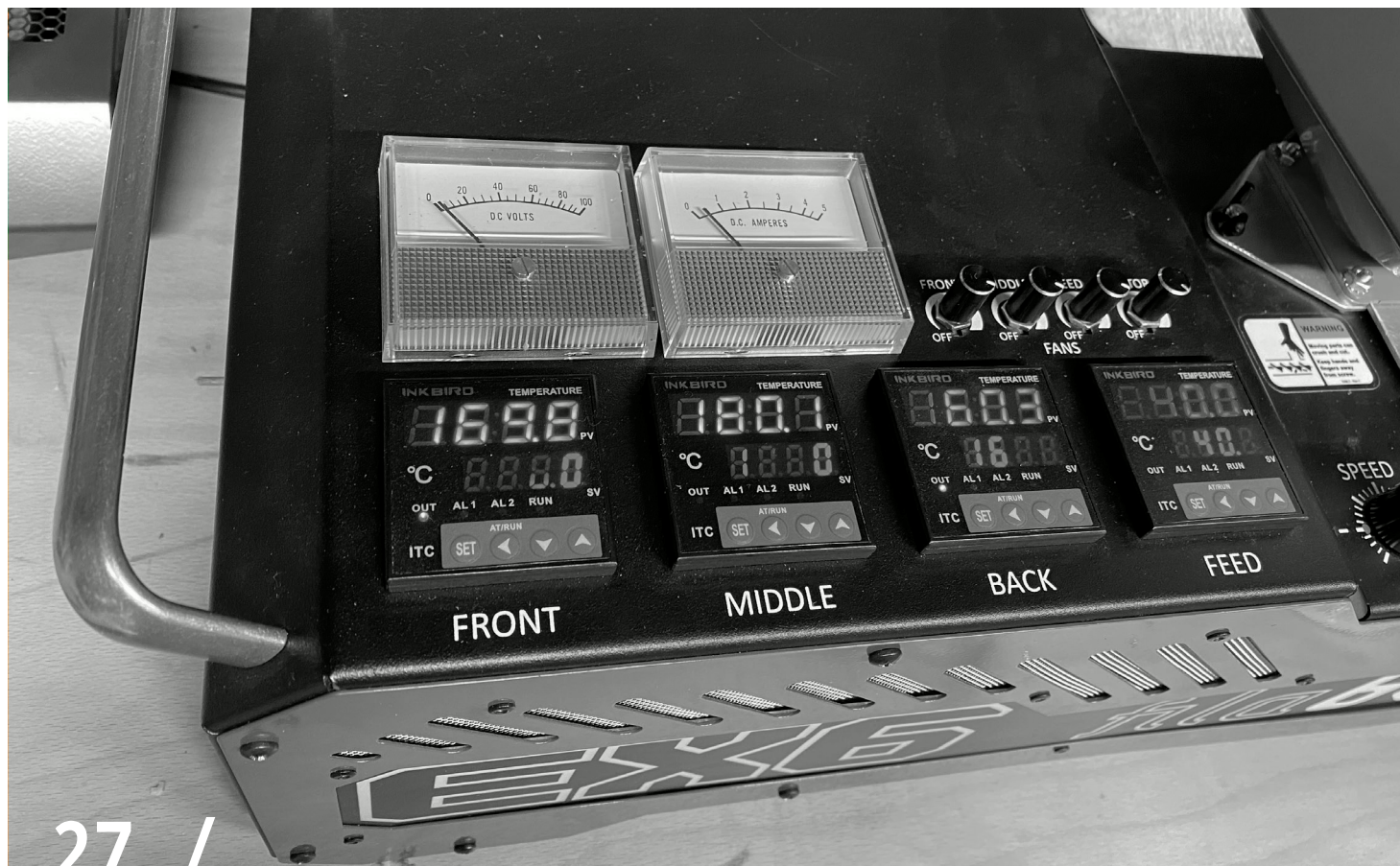
▲ Figure 27: Temperature Profile/ Temperature profile used to extrude the different materials on the 'Filabot EX6'. 169°C_180°C_160°C_40°C
