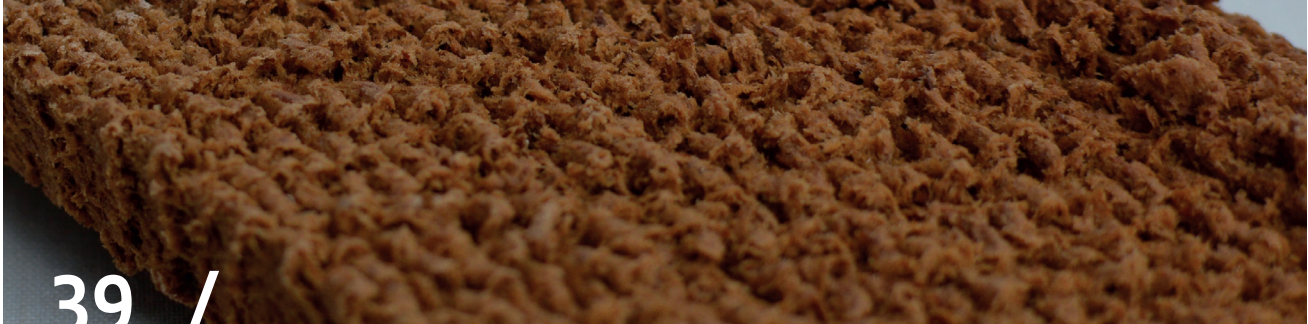
Figure 39: Rough Printed Surface/ ► Close up from the surface of WFPP that was printed.
