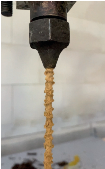
Figure 37: Rough Surface/ ▼ Representation of the fracturing of the surface for different materials when printing (50/50 mixture and WB60).
