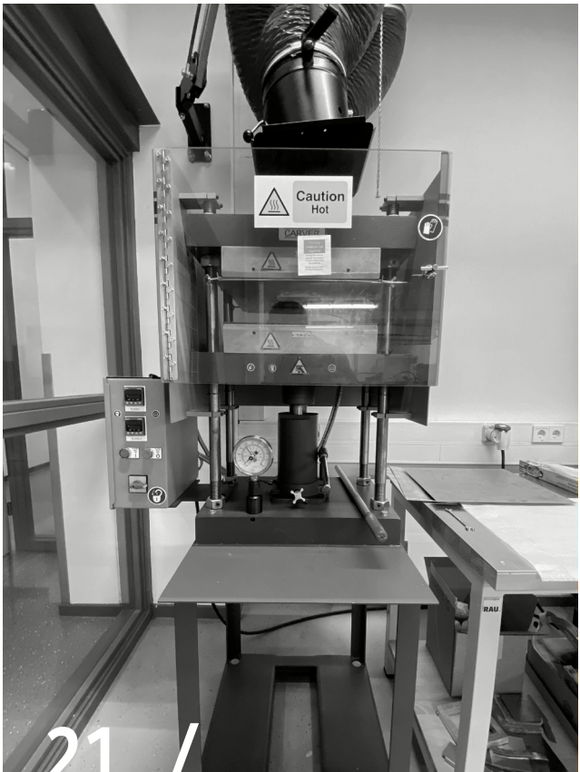
Figure 21: Heat Pressure Plates/ ▶ Press with heated plates to produce flat sheets from the granulate.
