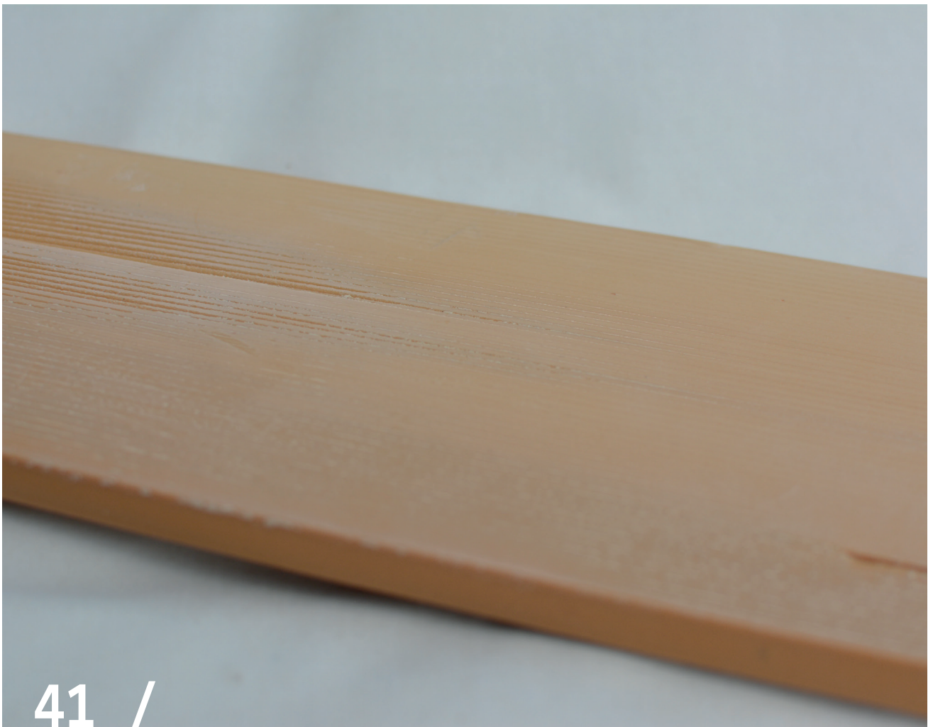
Figure 41: Smooth Surface Print/ ► CFPP sanded down with an eccentric sander and grain P800.
