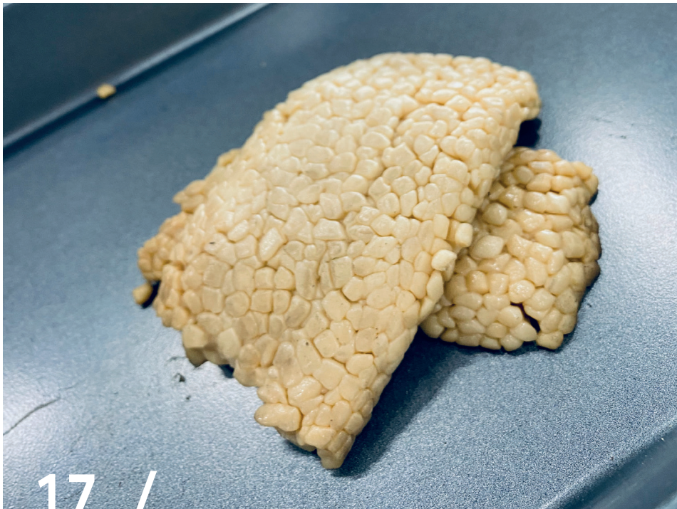
◀ Figure 16: PP with softwood/ Polypropylene with MFI 50 mixed with softwood chips.
