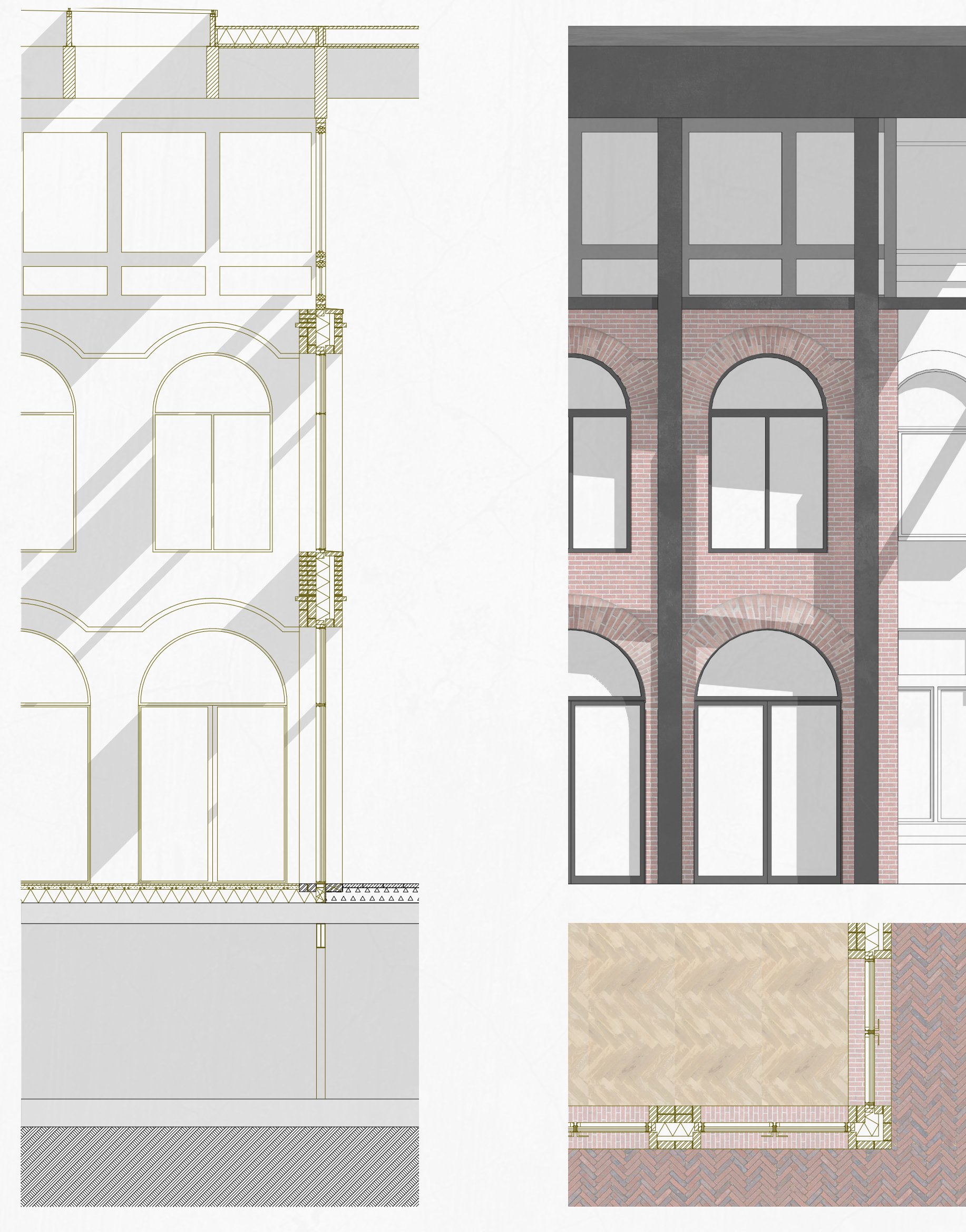
1:50 Facade section - new facade/entrance south cluster
