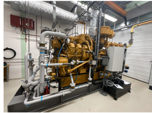
Fig. 1. The marine four-stroke spark ignition engine in the lab.
