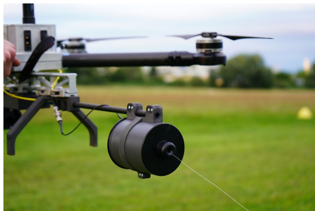
Figure 10.3: A spool with fiber optic cable, attached to a drone 1 .
