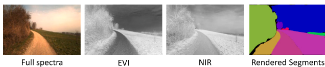
Fig. 9. Spectral renderings and rendered segments of the Freiburg forest dataset (Valada et al., 2016) with enhanced vegetation index (EVI) and near-infrared (NIR) components for a specific camera viewpoint.
