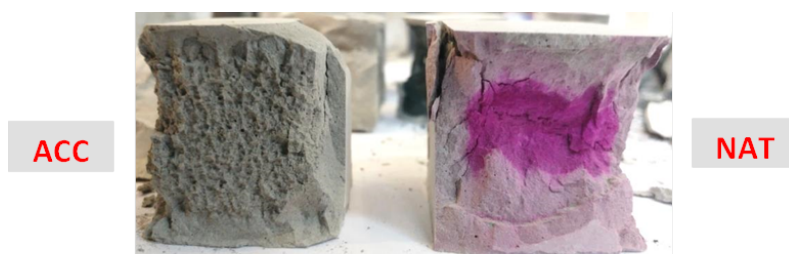
Figure 8.10: Appearance of the sample S30 after compressive strength tests. Left: sample surface eroded by accelerated carbonation, right: sample's surface exposed to natural laboratory carbonation.
