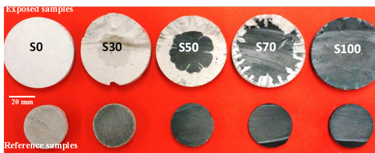
Figure 8.13: Cross-sections of representative samples after natural laboratory carbonation of 1 year, clearly showing the outer (carbonated) and the inner (noncarbonated) zone. Reference samples are of smaller diameter, placed beneath the exposed samples.
