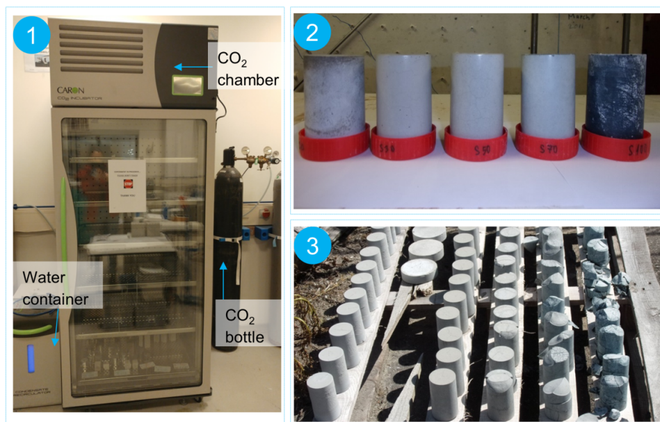
Figure 6.3: Exposure sites: (1) CO 2 chamber for accelerated carbonation, (2) natural indoor conditions, (3) natural outdoor conditions.
