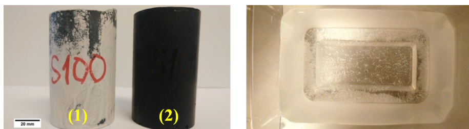
(a) Pastes S100 at 56 days (left, (1)-unsealed cured sample, (2)-sealed cured sample), the plastic container in which the fluid, condensed on the surface of the specimen S100, was collected after 4 days of unsealed curing (right).
