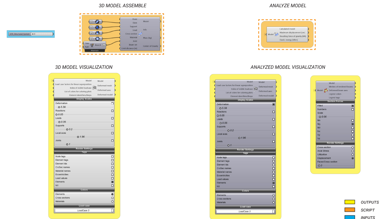
Figure 75. Script utilized to assemble and analyze the 3D model of the roof structure in Karamba 3D (Source: Self-made)
