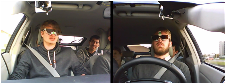
Fig. 2. Passenger and driver equipped with minimally invasive eye-tracking glasses.
