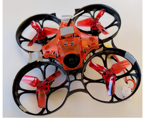
Figure 1. The black box equipped 75mm, 56g Tiny Whoop used during experiments
