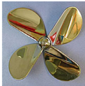
(b) Propeller used in the spherical combustion chamber used to generate a homogeneous isotropic initial turbulence field.
