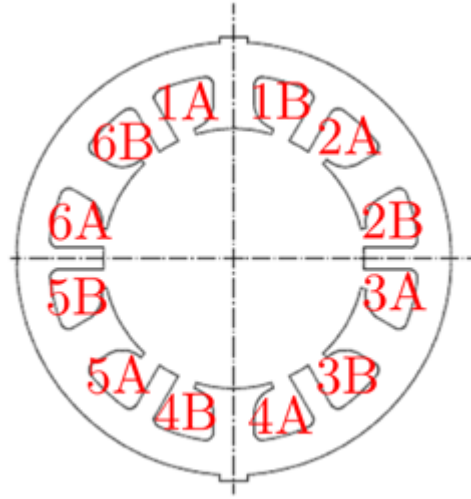
Figure 2.1: Machine stator winding structure
