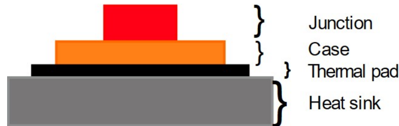
Figure 2.17: Thermal heat dissipation structure of To-263 SiC MOSFET
