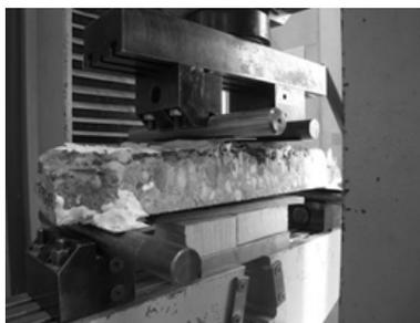
Figure 5.2: Test set-up used for four-point loading flexural tests.
