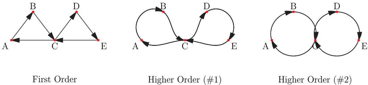
Fig. 2. A graph representation of a state transition sequence. The leftmost figure uses classical first order transitions, making it impossible to distinguish the sequence  $ABCABCABC\dots, CDECDECDE\dots$  from the sequence  $ABCDECABCDECA\dots$ . The rightmost figures take into account higher-order transitions to visualize the order in which the state transitions occur.
