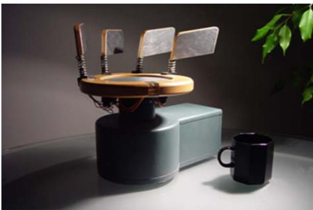
**Fig. 7** With the Carrousel, a tangible interaction device, users can "sculpt" atmospheres. The stage rotation speed and the orientation of the flags can be changed to express a desired atmosphere
