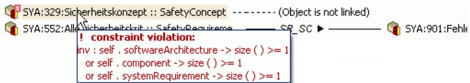
Fig. 8. Evaluation of an OCL constraint in ToolNet.
