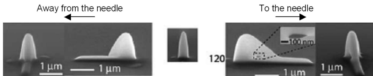
FIG. 30. The effect of the writing direction with respect to gas nozzle. A tip was deposited, followed by a line deposition. When the line was written away from the nozzle, significantly less material was deposited than when the line was written toward the nozzle. From Ref. 129. Copyright © 2005 by Elsevier. Reprinted with permission by Elsevier.
