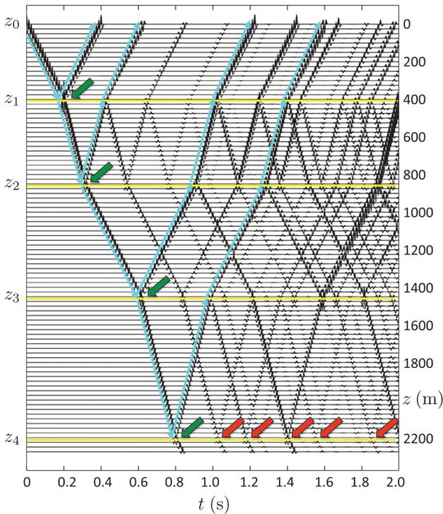
Figure 1. Retrieved Green’s function  $G(z, z_0, t) * s(t)$ . The imaged reflectors in Figure 2a come from the first arrivals in the down- and upgoing Green’s functions just above these reflectors, indicated by the green arrows.
