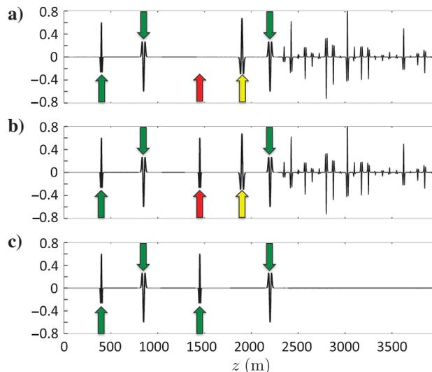
Figure 4. Marchenko event-by-event deconvolution images obtained from the reflection response, which misses the primary of the third reflector. (a) Image obtained from the primaries. (b) The same, but including the image of the third reflector, obtained from the multiple indicated by the red rays in Figure 3. (c) Image obtained after restoration of the primary response of the third reflector.
