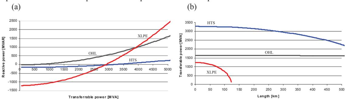
Fig. 2. (a) Reactive power as function of the active power flow for 33.8 km long connection: OHL (black), XLPE (red) and HTS (blue) cables. (b) Transmittable active power as function of the connection length for  $\cos\phi = 1$ : OHL (black), XLPE (red) and HTS (blue).
