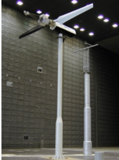
Figure 3.1: The NREL phase VI turbine in the NASA Ames wind tunnel [30].
