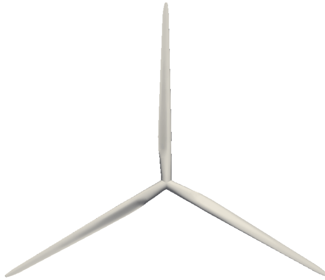
Figure 3.2: The NREL 5MW turbine rotor geometry.
