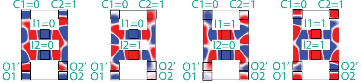
FIG. 4. Fan-in of 2 AND/OR Gate OOMMF Simulation
