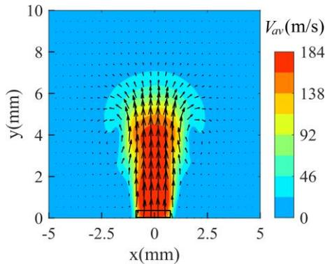
Fig. 3 Typical phase-averaged velocity field for Case 3. Elapsed time from ignition of discharge is  $t = 150 \mu s$ . Black rectangle above exit indicates the interrogation window. See Fig. 1 for the definition of coordinate system.
