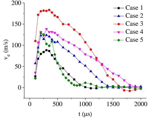
Fig. 4 Phase-averaged exit velocity in one period.
