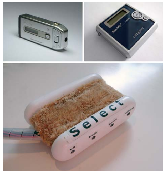
Fig. 2 Top Regular MP3 players are operated by buttons, (touch-sensitive) scroll wheels and sliders. Bottom Puppy, a MP3 player to reduce stress, is operated by stroking where the place, direction and character of the stroke determine how the functionality is processed and executed (designed by Master student Johannes Zachrisson for the course Interactive Technology Design at the Delft University of Technology)
