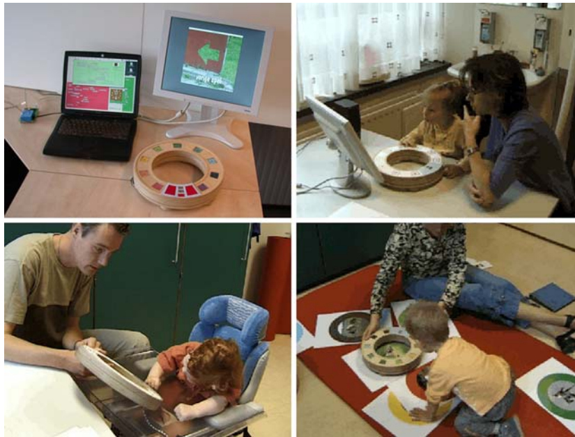
Fig. 3 Explorascope is an interactive educational toy for multi-handicapped children. The complexity and possibilities of the stories, the interaction and the configuration can be adjusted to an individual child. For example, Child1 prefers moving the E-scope over the table, turning the upper ring and pushing the Picture Communication Symbols (PCS) on the wooden ring to
