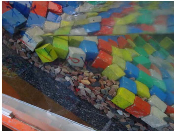
Figure 39: Removed concrete blocks and extraction of the underlayer
