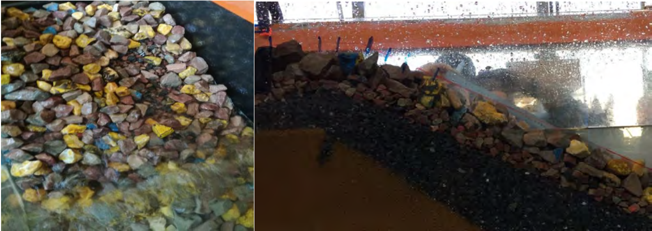
Figure 14: Damage observed on the wave flume model
