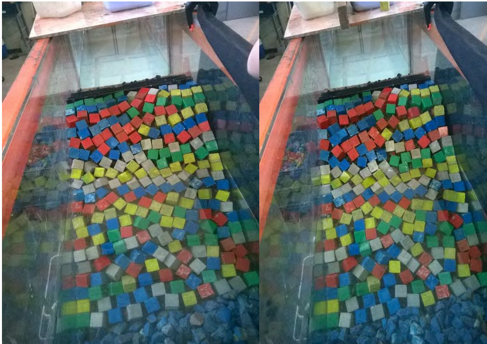
Figure 40: Before and after the test. In the second picture it can be seen the sliding of the armour layer.
