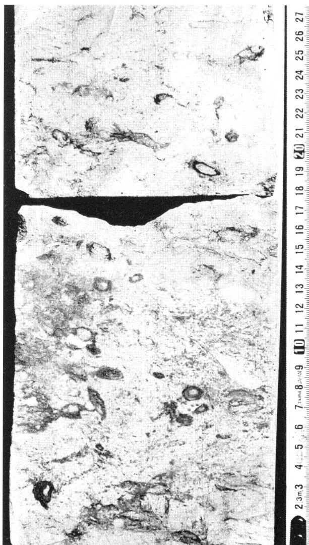
Fig. 2. Core photograph of the Rijn Member. Bioturbated very fine sand with abundant Asterosoma . Well B-1, depth 1980.8 m.
