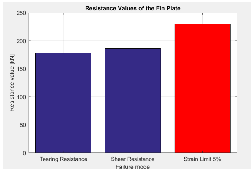
Figure 6.8: Comparison resistances values fin plate, EC3 and FEA model
