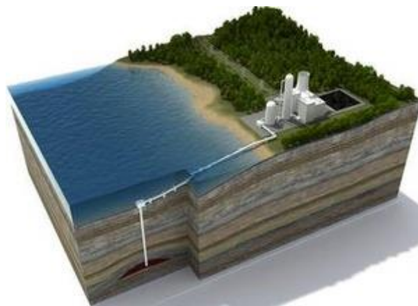
Figure 1.9: Power plant equipped with Carbon Capture and Storage (CCS). Power plant equipped with pre- or postcombustion carbon capture process, transportation pipeline and underground CO 2 storage facility.
