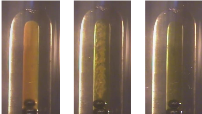
Figure 1.7: Experimental setup: Cailletet tube (including magnetic ball stirrer). Phase transition from nematic phase (left) to isotropic liquid phase (right)
