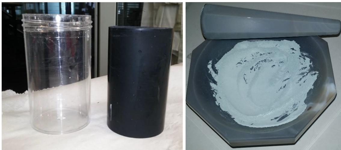
Fig. 5 Bulk sample after demolding (left), and ground sample (right) (Color figure online)
