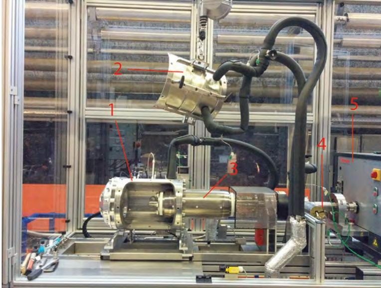
Figure 5.2: Actual picture of the Up-Scaled Couette Cell. 1. Housing; 2. Lid; 3. Inner cylinder; 4. Shaft; 5. Rheodrive unit.
