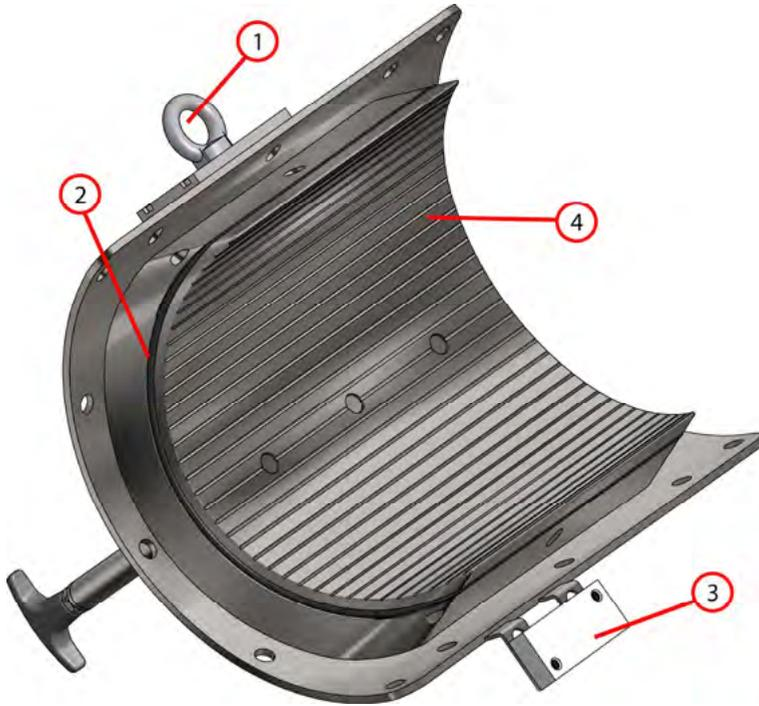
Figure 4.8: Back of the up-scaled Couette Cell's lid. 1. Hook 2. O-ring seal 3. Magnetic safety plug 4. Corrugations
