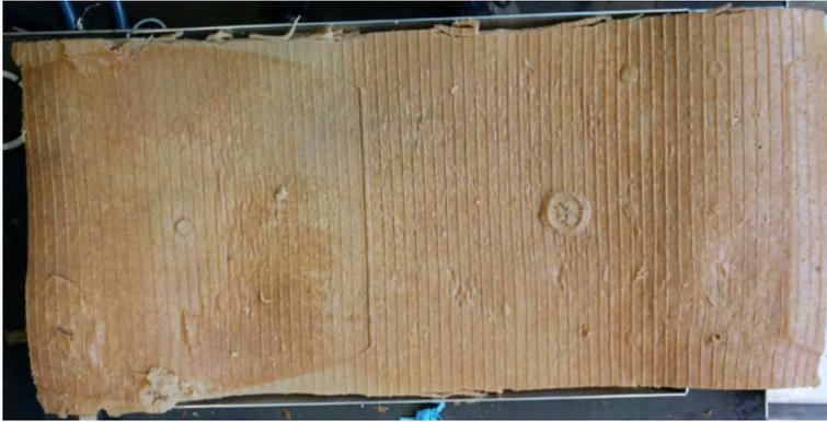
Figure 5.4: Typical product slab obtained at 120 °C, 20 RPM and 30 minutes (Length = 596 mm, Height = 332 mm).
