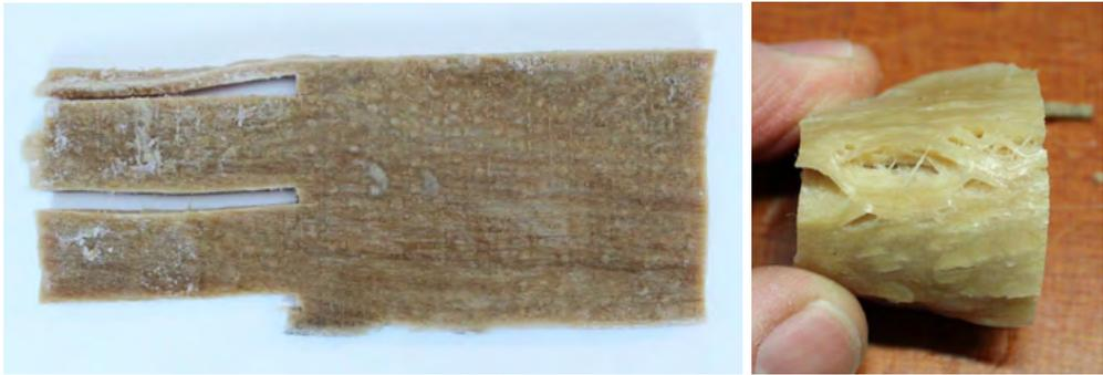
Figure 2.5: Samples displaying fibres. Left: View of the sample when frozen; the fibres are more visible; notice the sample cuts on the left. Right: Details of sample displaying fibrous structures. This sample was created at 95 °C, 30 RPM and 15 minutes of process time.
