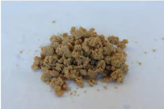
Figure 2.3: The SPI - gluten - demi-water - salt mixture before it is filled in the Couette Cell.
