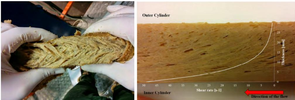
Figure 5.3: Left: Typical fibre structured sample obtained at 120 °C, 20 RPM and 30 minutes. Right: Sample thickness (30 mm). Notice the structure formation following the flow direction and the similar pattern of the shear rate profile across the thickness as calculated by Equation 5.6.
