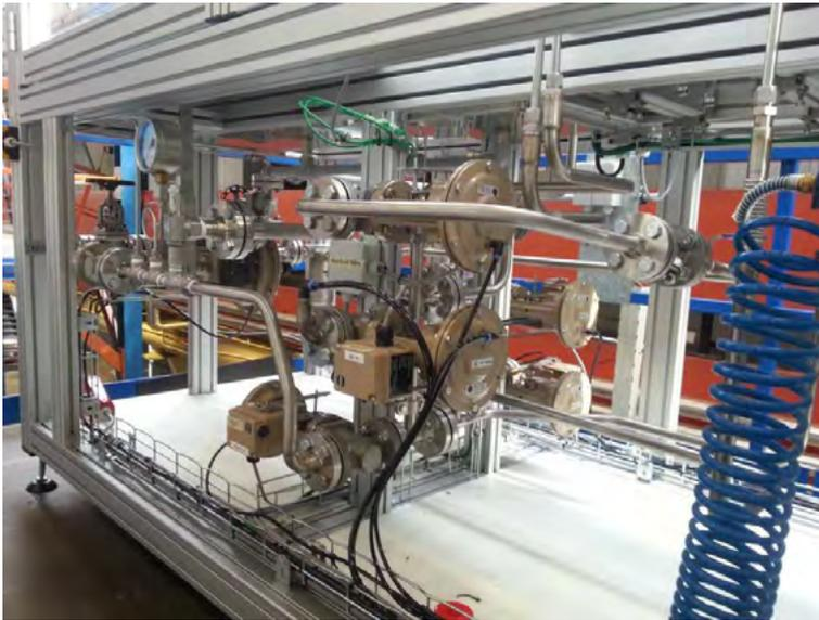
Figure 4.12: Picture of the control hardware used in the up-scaled Couette Cell.
