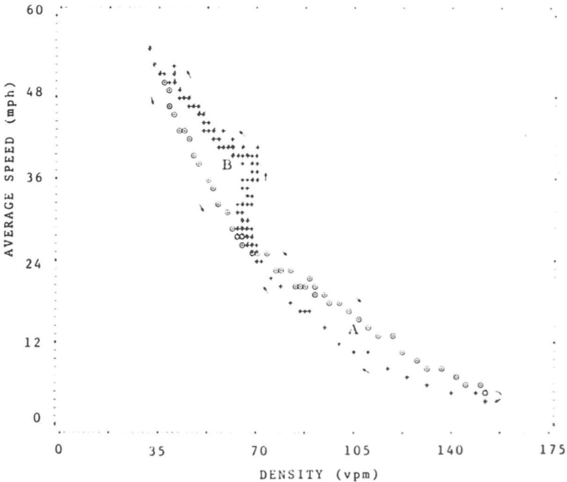
**FIGURE 6** Observed densities and speeds showing the hysteresis phenomenon. At relatively low densities, speeds are higher when accelerating (diamonds) than when decelerating (circles), at relatively high densities, it is the other way around. Picture from [11].
