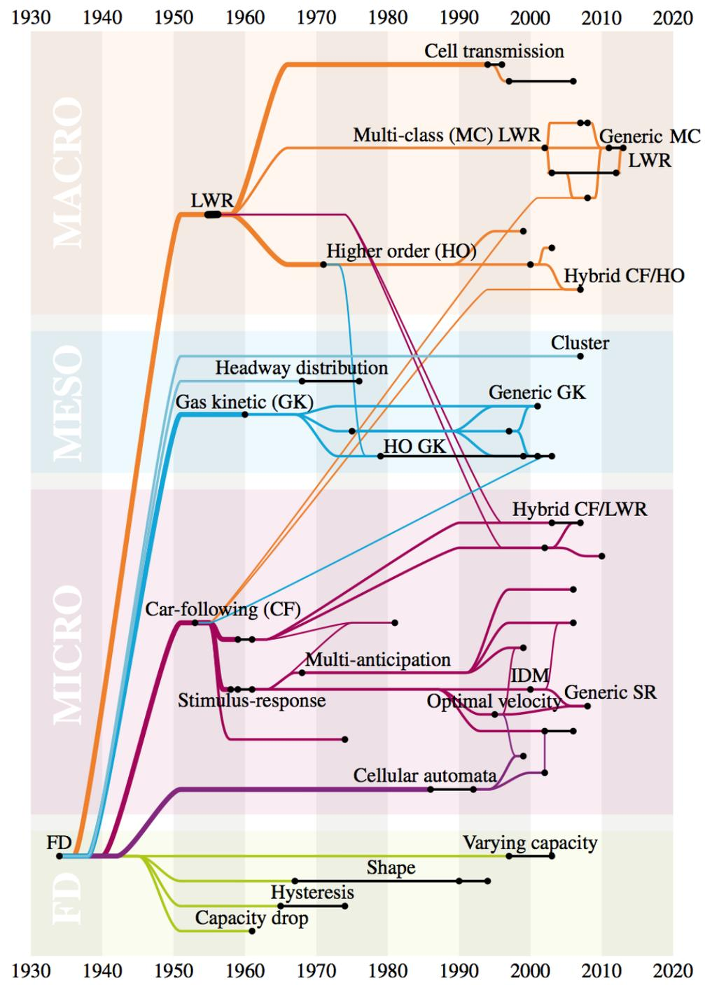
**FIGURE 1** Genealogy of traffic flow models. Black dots indicate models, black lines between dots indicate that the same (or a very similar) model has been proposed multiple times, colored lines indicate descent. A full (and much larger) version of the genealogy can be found in [63, 75].
