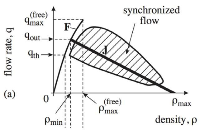
**FIGURE 7** Fundamental diagram with infinitely many admissible states in the congestion branch (shaded area). Picture from [77]. For detailed explanation of the labels, we refer to [77].
