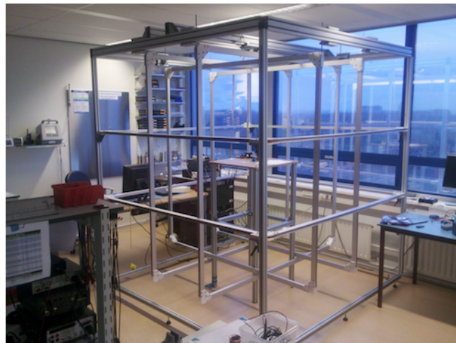
Figure 7-1: The Helmholtz cage located in the clean room.
