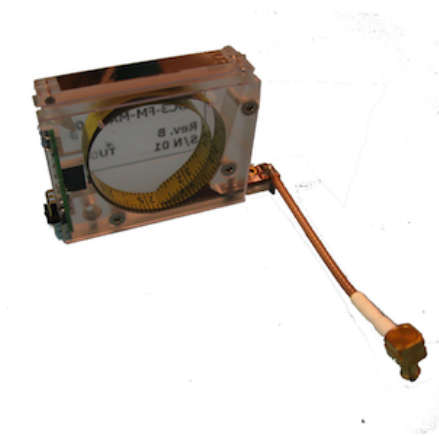
Figure 2-16: A Modular Antenna Box with an antenna rolled up inside
