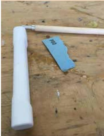
9. The rest of the parts are printed. This is done because it allows for more accurate painting later.
