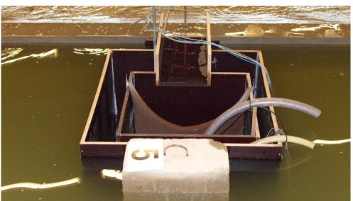
Fig. 3.8.: Overtopping box with pumps and chute.
