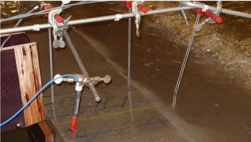
Fig. 3.9.: Three wave gauges and a propeller on the crest.
