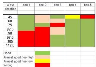
Fig. 6.1.: Overview of reliability of test results at overtopping boxes (Van der Meer, 2012a).
