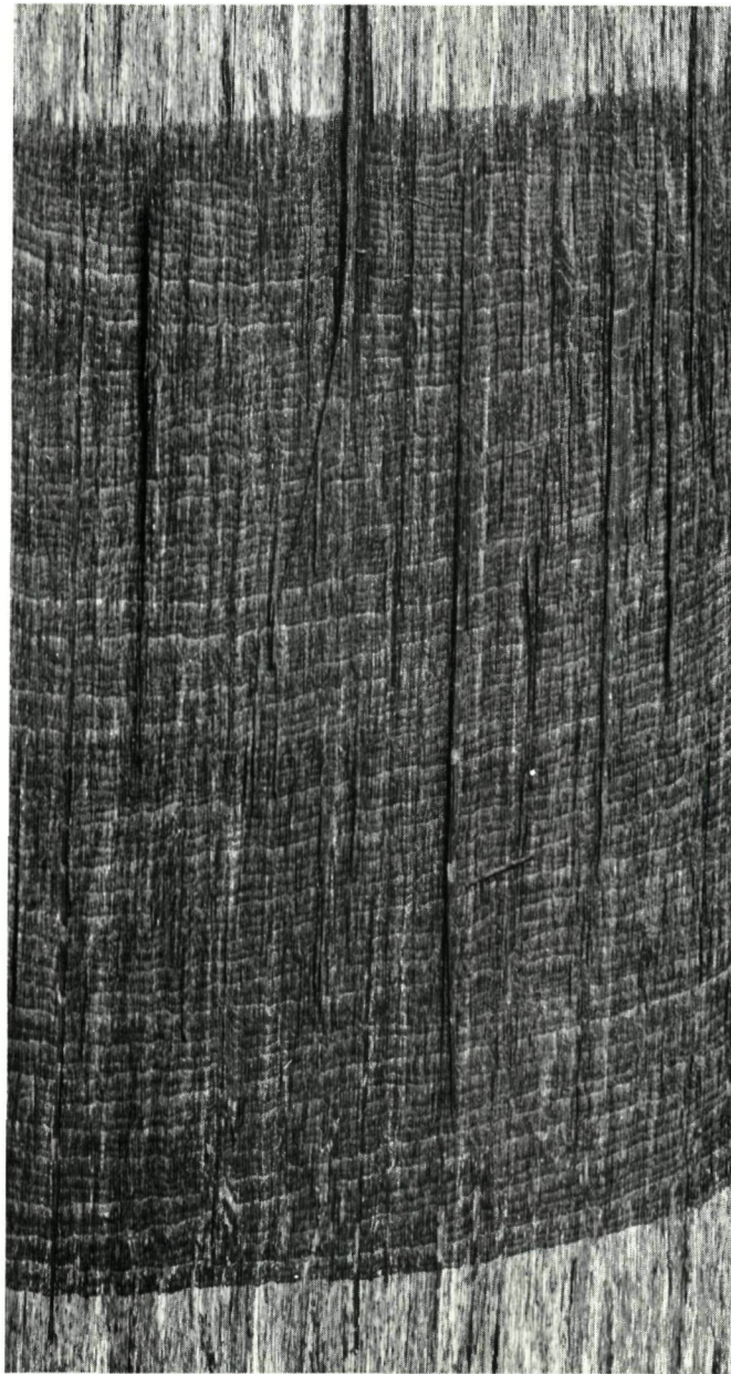
Fig. 14 Fracture surfaces of a DCB specimen
