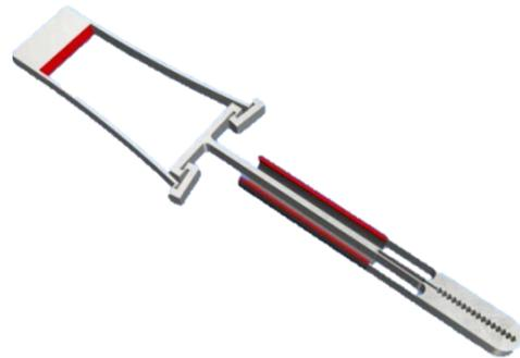
**Figure 14.** Statically balanced gripper with a perfect ratio between applied input and clamping force [16].
