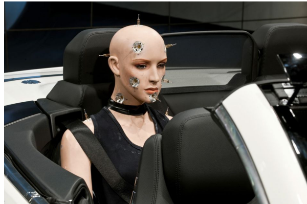
Figure 1.2: Measurement manikin to evaluate the thermal comfort in open cabriolets [9]
