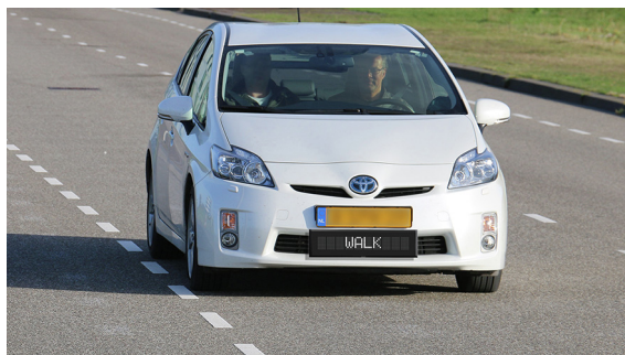
Fig. 2. One of the six eHMIs used in the experiment. The person in the driver seat provided written consent for the publication of this photograph.
