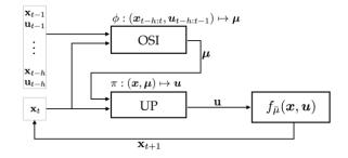
**Figure 4-2:** The Online System Identification provides a policy  $\pi$  to the controller that provides the action to the environment [3]
