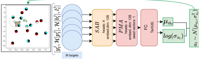
Fig. 2. Policy neural network architecture. The sequence of target information is fed to the self-attention block (SAB) which encodes and identifies how each target pose affects the visibility of the others from the drone’s perspective. This information is fed to the pooling multi-head attention layer (PMA) and mapped through a fully connected layer (FC) to obtain the policy viewpoint recommendation.
