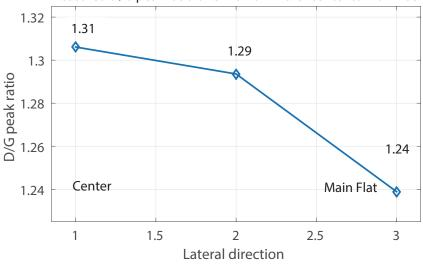
Measured D/G peak ratio of CNTs from wafer center to main flat
