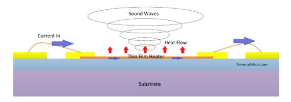
Figure 1.4: A simple schematic of the physics of thermoacoustics: Heat is generated by AC current and passed to the surrounding air causing pressure variation which is sound waves.
