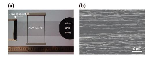
Figure 2.1: CNT thin film design [9], drawing and handling the CNT thin film is a difficult and delicate process which is not suitable for mass-production.
