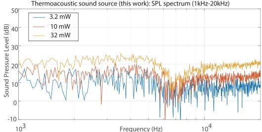
Figure 7.12: The SPL frequency response of thermoacoustic sound source (this work). The SPL response is noisy as shown due to the low sound pressure detected is near the self noise level of the Microphone.
