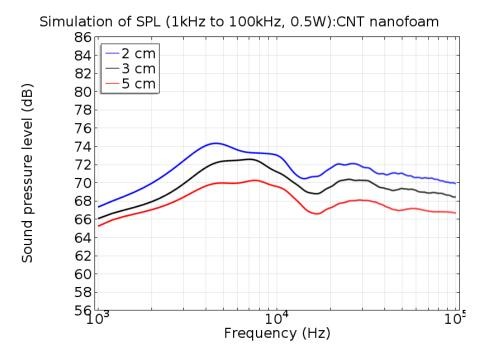
Figure 4.7: Simulative frequency response of SPL of CNT nanofoam device from 1 kHz to 100 kHz at a input power of 0.5 W
