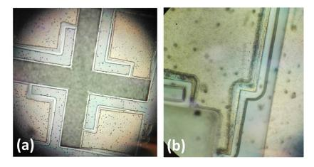
Figure 6.5: The accelerated HF vapor etch due to water accumulation, viewed under optical micro scope.
