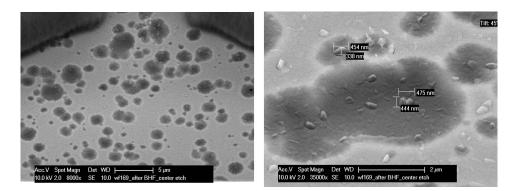
Figure A.7: SEM images of damages on TiN layer, black dots. This damage is not catastrophic, CNTs can still grow on the TiN if the dots density is not too high, however the growth on the dots are largely affected which can result in doted pattern in the grown CNTs as well.
