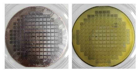
Figure A.5: (Left), wafer with 1 um thick SiC masking layer after CNT growth which is cracked all over the wafer, (Right), Bad adhesion of photo-resist after long steps of dry-etching on SiN masking layer
