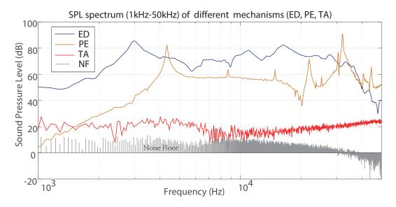
Figure 7.13: Comparison of ED,PE and TA SPL vs frequency (1 kHz to 50 kHz), the SPL frequency response show a wide band flat behavior
