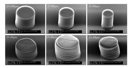
Figure 3.4: SEM images of compressed CNT nanofoam in different diameters [34].
