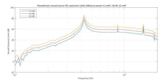
Figure 7.11: The SPL frequency response of piezoelectric sound source, at power of 3.2 mW, 10 mW and 32 mW. Piezoelectric mechanism result in multiple resonance peaks and low performance at low frequency range.
