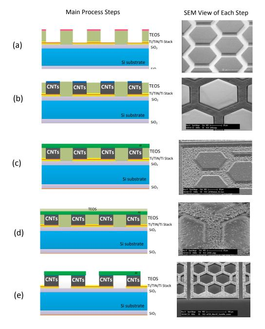
Figure 5.2: The schematic of main process steps and its correlating SEM images.
