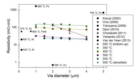
Figure 3.3: Resistivity of bundles obtained at different temperature and catalyst [38].
