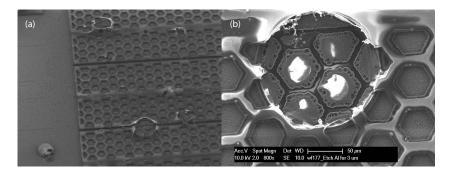
Figure A.4: The bubbles inside photo-resist that are produced by the air expansion from CNTs when heated, it is catastrophic issue since re-coating requires removal of the photo-resist, either plasma striping or ultrasonic bath in NMP to remove photo-resist can damage the CNTs. It is recommended to put thick enough TEOS oxide to seal 100% before coating
