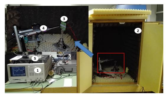
Figure 7.9: A demonstration of the measurement setup used to characterize acoustic performance of sound sources
