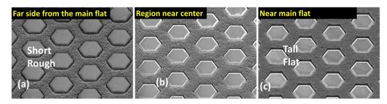
Figure 7.3: Non-uniformity of CNT growth over wafer scale
