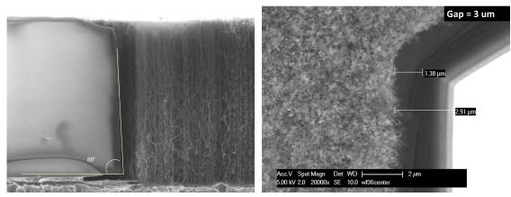
(a) Cross-section profile of the etched side wall of TEOS oxide
