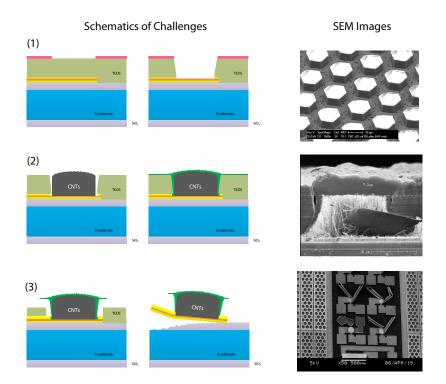
Figure 6.1: Critical steps that lead to challenges in fabrication
