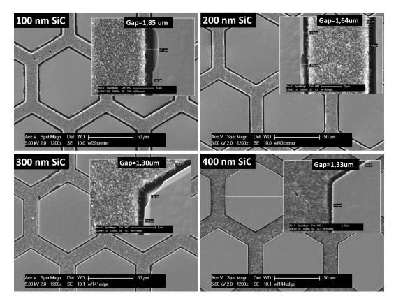
Figure 6.8: Different thickness of SiC masking layer, 100 nm, 200 nm, 300 nm and 400 nm, used to close the CNT-TEOS gap
