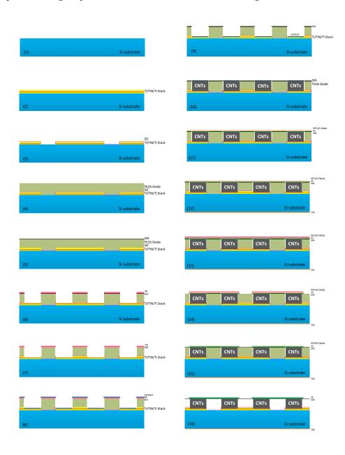
• The optimized design of process flow to solve the encountered challenges:
