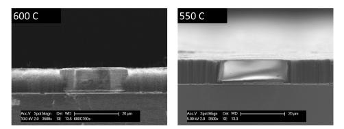
$\label{eq:constraint} Figure A.10: CNTs grown at 550\ ^\circ C and 600\ ^\circ C, 550\ ^\circ C result in more uniform height of CNTs, and 600\ ^\circ C gives a more aggressive growth and less accurate and conformable height control.$
