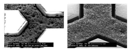
Figure A.8: (left), non-uniform growth caused by dots on TiN layer, as observed that the height of CNTs at the dots are much lower and result in holes in the nanofoam, (right), the desired flat and uniform CNT nanofoam grown on good quality TiN.
