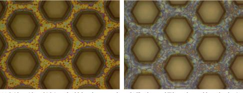
(a) Oxide residue which is preferablely to be removed completely in the TEOS oxide dry etching, since the residue can increase the time to remove all Ti sacrifial layer beneath which can enlarge the TEOS-CNT gap.
