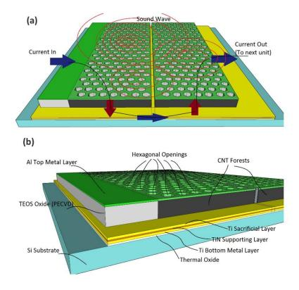
Figure 3.6: A 3D model of our proposed CNT nanofoam design with hexagonal openings for sound emission. (a) Zig-Zag current created by vertically conducting CNT arrays, heating causes air expansion and result in sound emission from the openings. (b) Side view of applied materials in the design.
