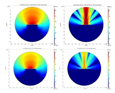
Figure 4.8: Simulative frequency response of SPL of CNT thin film device from 1 kHz to 100 kHz at a input power of 0.5 W
