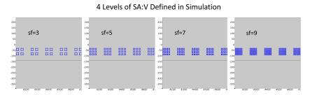
Figure 4.2: An illustration of heater units with different surface area to volume ratio used in the simulations.
