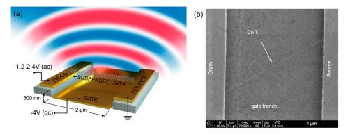
Figure 2.4: Single suspended CNT TA device [26] is scientifically the smallest acoustic unit measured, however not suitable for consumer application.
