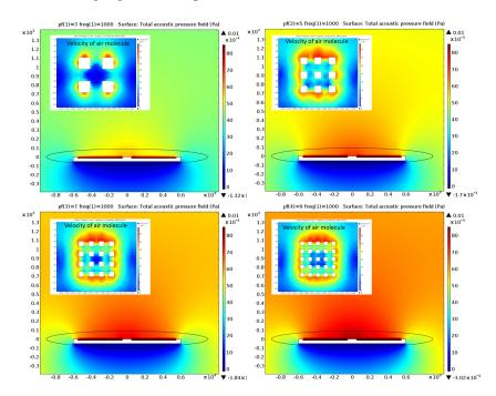
Figure 4.3: Total pressure field (large) and velocity of air near heater (small) at different surface area to volume ratio.
