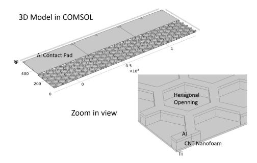
Figure 4.9: The 3D model built in COMSOL to evaluate the current distribution of the nanofoam design
