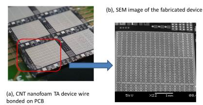
Figure 5.1: The fabrication result of our proposed processing approach
