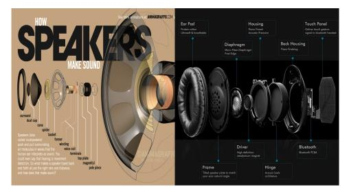
Figure 1.2: An anatomic view of speaker and headphone, the latest designs of bluetooth headphones still employs electrodynamic acoustic drivers. [1, 2] Thermoacoustics sound source can be potentially integrated on to a chip with other electronics.
