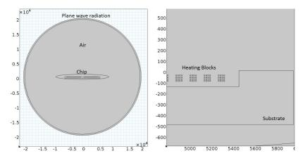
Figure 4.1: 2D Model for thermoacoustic simulation: simulation for different surface area to volume ratio.
