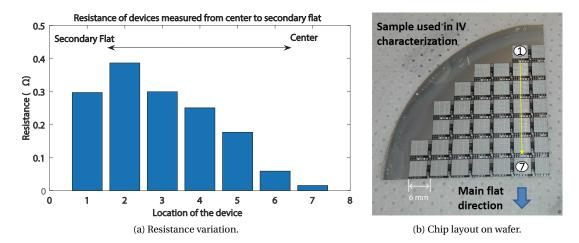
Figure 7.7: The resistance variation from wafer center to edge.
