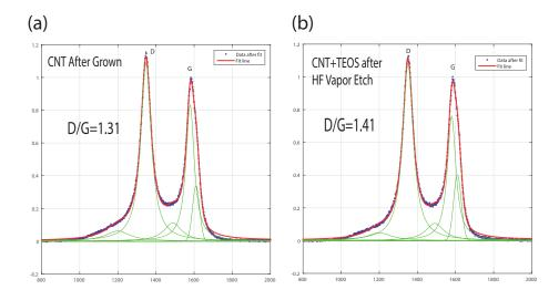
Figure 7.1: Raman spectrum of CNTs at two different process steps, as grown and after HF vapor etch.
