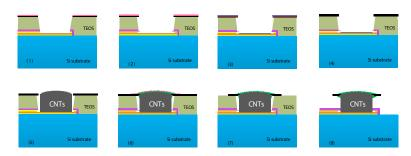
Figure 6.2: Optimized processing steps to solve the challenges: SiC protection layer for bottom Ti metal pad and masking layer on top of TEOS oxide to close the gap
