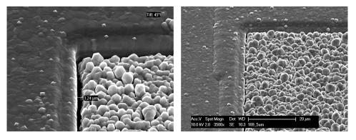
Figure A.9: SEM images showing 3 um Al sputtered on CNTs (left) and 5 um Al sputtered on CNTs (right), this shows the step coverage is not sufficient to close the TEOS-CNT gap and pinholes. It is expected from the images that 10 um Al is required to obtain uniform surface.
