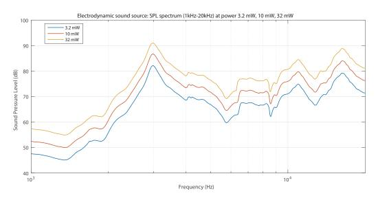
Figure 7.10: The SPL frequency response of a commercial electrodynamic sound source from 1 kHz to 20 kHz at different power levels, 5 dBm (3.2 mW), 10 dBm (10 mW) and 15 dBm (32 mW). SPL increases linearly with the input power (dBm).
