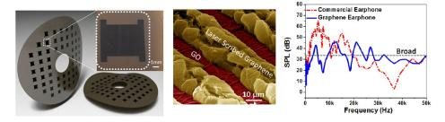
Figure 2.5: TA design with reduced graphene oxide [15]. Large peaks exits in the SPL frequency response. Fabrication requires laser scribing which is not suitable for mass-fabrication.
