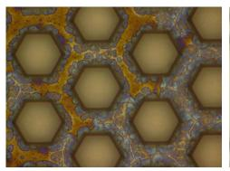
(a) Damaged Ti sacificial layer
