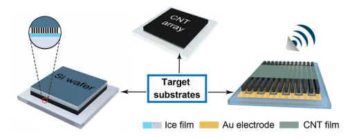
Figure 2.3: CNT thin film over laser patterned CNT arrays [24], extra complexity of fabrication with ice transfer, still lack ability of scaling down and mass-production.
