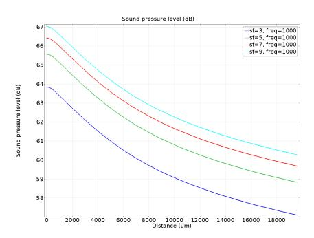
Figure 4.4: SPL vs distance away from the thermoacoustic sound source at different SA:V values.
