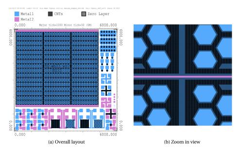
Figure 5.4: Mask designed for the process, consist of 3 different images in black(CNTs), blue(Metal-1) and pink(Metal-2).
