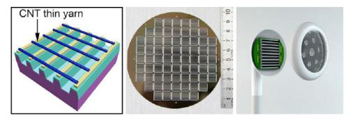
Figure 2.2: CNT thin yarn design [10], fabrication of CNT thin yarn requires transfer of CNT thin film, laser patterning and atomization which is not efficient and low scalability.
