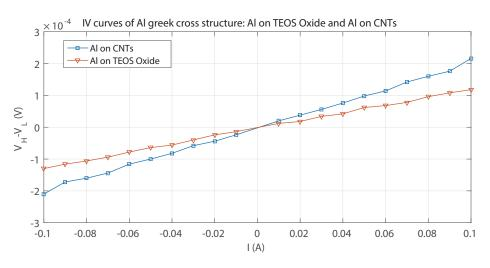
Figure 7.5: The I-V curves of the Al greek cross structure both fabricated on TEOS oxide and CNT nanofoams
