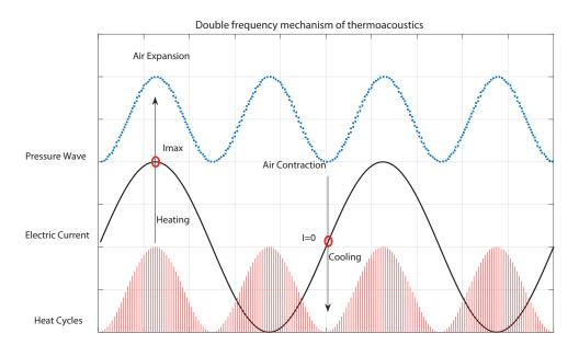
Figure 1.5: The mechanism of double frequency effect in thermoacoustics.
