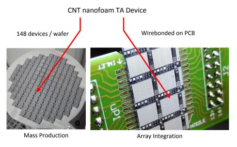
Figure 5.3: A view of the fabricated devices on a wafer and assembled on a PCB. It shows the ability of mass production and integration of our CNT nanofoam design.
