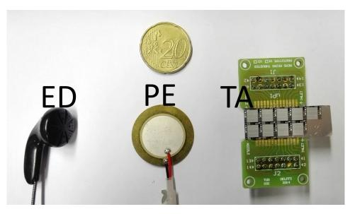
Figure A.11: Devices under test in the acoustic measurement, from left to right is the electrodynamic device, piezoelectric device and our TA device. They have approximately the same device area.
