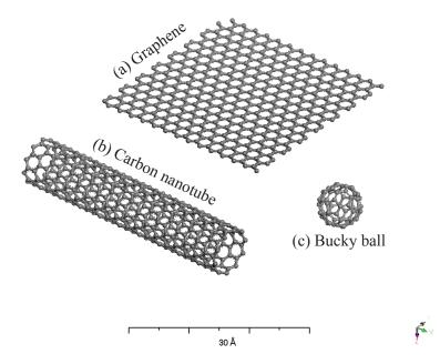
Figure 3.1: (a) Illustration of graphene showing a single layer of carbon atoms in a honeycomb lattice, the material is considered to be two-dimensional (2D). Multiple layers of graphene stacked is called graphite. (b) The rolled up version of the single or multilayer graphene sheets are called single- or multiwall carbon nanotubes, respectively, and they are considered to be 1D. (c) The last example shows a Buckminsterfullerene C60 which is considered to be a 0D material
