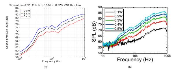
Figure 4.6: Validation of the COMSOL model by matching to literature: (a), Frequency response of a CNT thin film TA speaker at input power of 0.5 W based on our COMSOL model and (b) the measurement result from literature [24].
