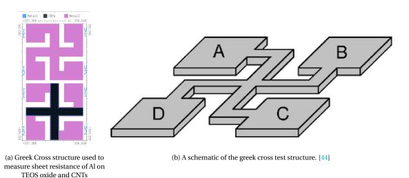
Figure 7.4: Greek test structure for measuring the sheet resistance of Al in the fabricated device.
