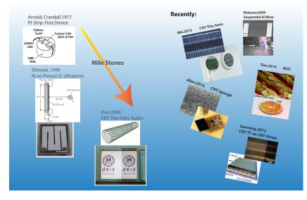
Figure 1.3: The Development of Thermoacoustic Sound Sources, the discovery of CNT thin film as thermoacoustic heater is the mile stone for recent development of thermoacoustic designs.
