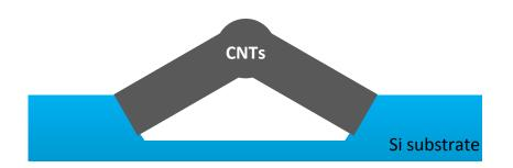
Figure 8.1: Self connection made by as grown CNT bundles, in this way further top metalization is not needed
