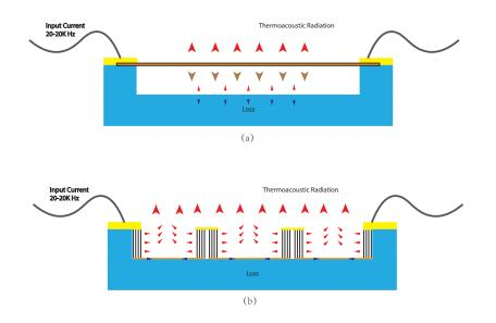
Figure 3.5: Illustration of the difference between 2D and 3D design. (a) Illustrates the 2D design and the less optimal orientation of acoustic emission. (b) Our proposed 3D solution.
