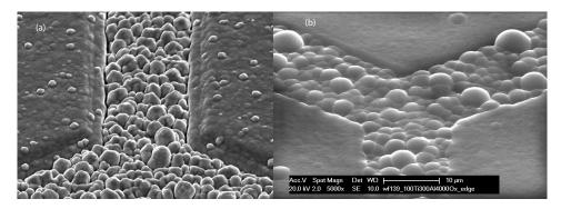
Figure 6.9: A comparison between the ability of Sputtered Al and PECVD oxide to seal gaps and pinholes. a),With 5 um Al sputtered on CNTs. b),With 4 um PECVD oxide deposited on CNTs
