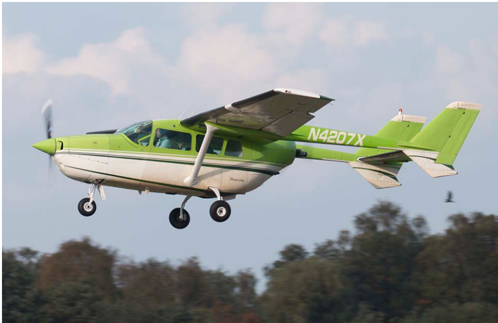
Figure 2.1: The Cessna 337F Skymaster which shall become a flying test bed for sustainable aviation.
